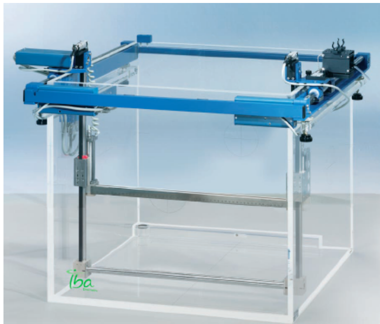
Figure 3-2: The 3D water phantom system (Blue Phantom) used for beam profile and PDD measurements [5].
