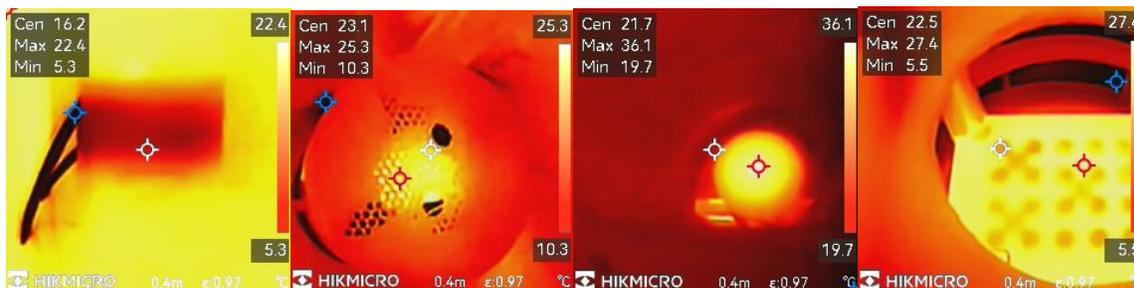
**Figure S4.9:** Thermal imaging measurements of the photoreactor attached to recirculation tubing (far left), the top of the photoreactor, showing electronic components and motor inside (center left), the fan and interior of the lamp holder (center right), and the inner chamber showing the reaction block bottom (far right).
