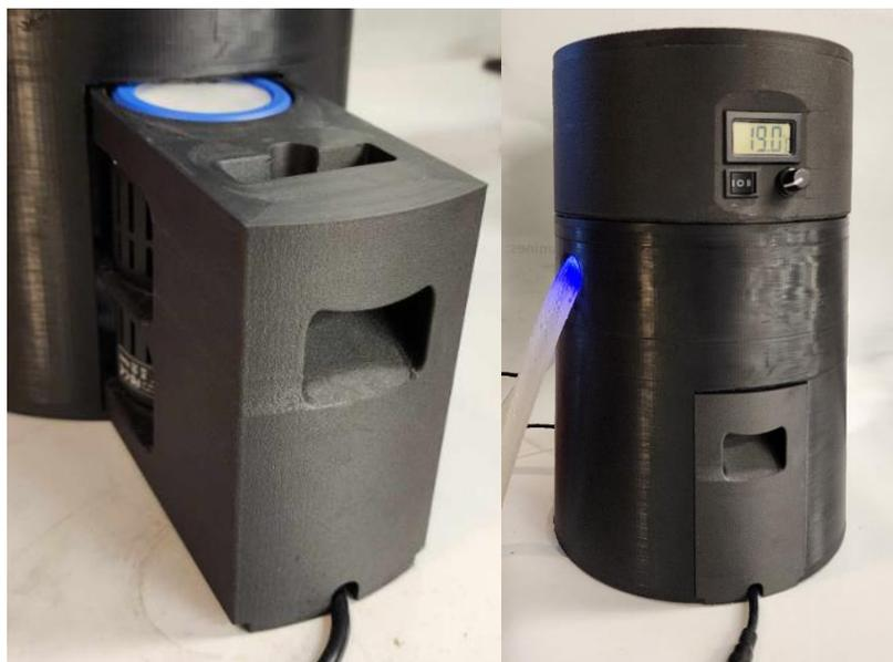
**Figure S4.7:** Placement of the lamp within the drawer (Left, note that it includes a pocket for filter storage). Fully assembled photoreactor (right).
