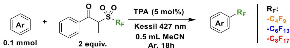
**Scheme S3.1.** The aromatic substrate (0.1 mmol), the corresponding perfluoroalkylating reagent (0.15 – 0.2 mmol, and 0.005 mmol of triphenylamine were added into 0.5 mL acetonitrile inside a glass test tube capped with a rubber septum. Three freeze-pump-thaw cycles under argon were carefully performed before setting the reaction under light irradiation at 20°C using a Kessil PR160L 427nm (45W) LED lamp. Two desk fans were
