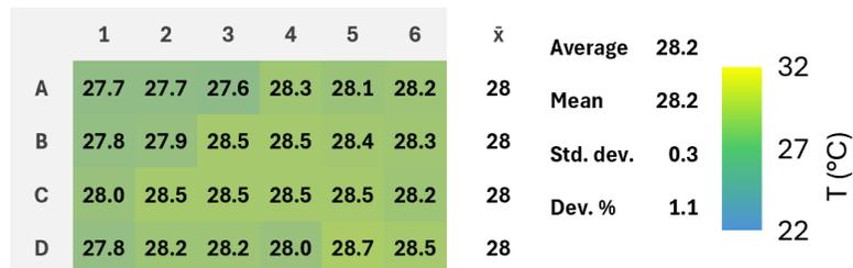
**Figure S4.11:** Plate temperatures inside the reaction solution
