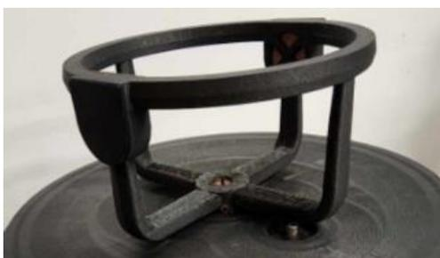
**Figure S4.2:** Fixed rotor piece in place. Note the thermometer sensor placement in the bottom.
