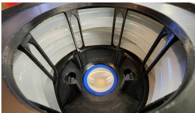
**Figure S4.4:** Interior of the photoreactor body bearing 6 tubing turns. Notice the lamp placement underneath (Always make sure to align and level the lamp before running reactions).
