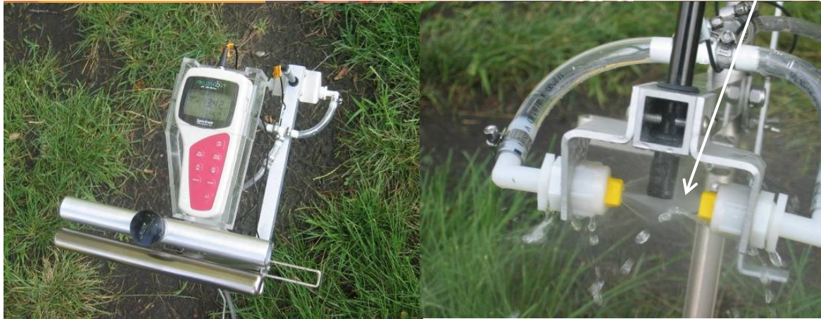
Fig. 3.2 Instrumented manual probe for on-the-spot soil ion measurements
