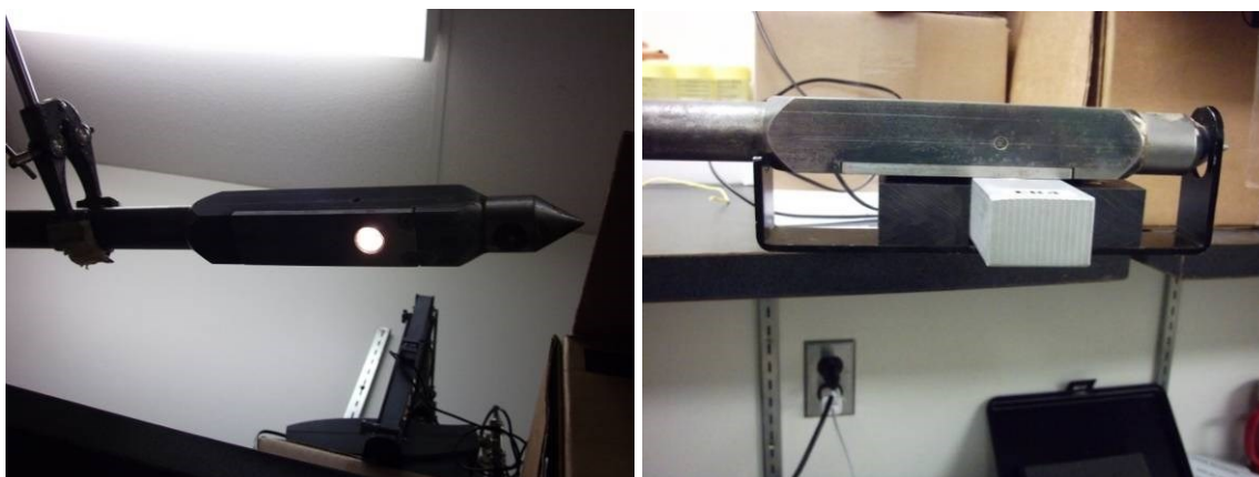
Fig. 6.3 Illustration of the vis-NIR soil profiling tool during laboratory measurements
