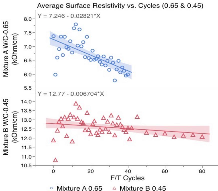
Figure 25: Average surface resistivity vs. cycles (w/c 0.65 & w/c 0.45)
