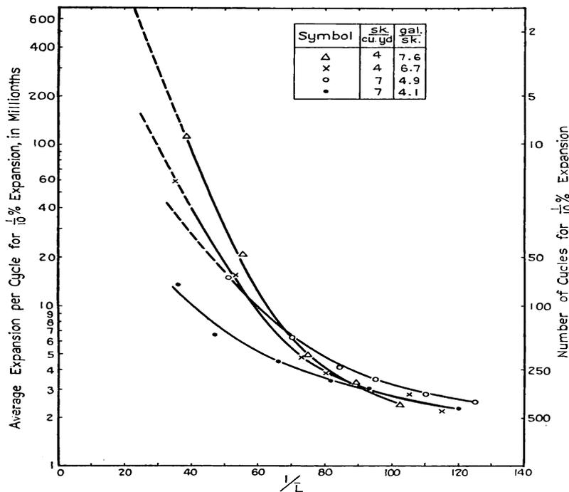
Figure 3: Relationship between frost resistance and spacing factor
