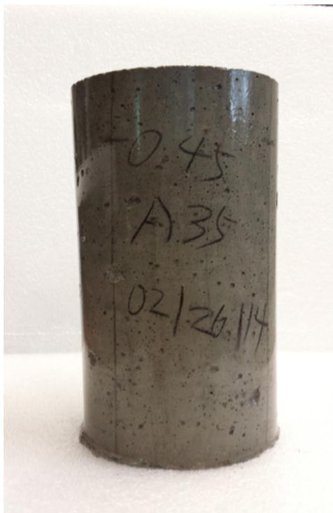
Figure 24: Specimen #35 of Mix 0.45 after subjected to 80 cycles.
