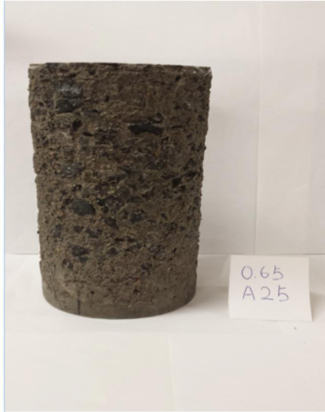
Figure 22: Concrete sample #25 of Mix 0.65 after 40 freeze-thaw cycles
