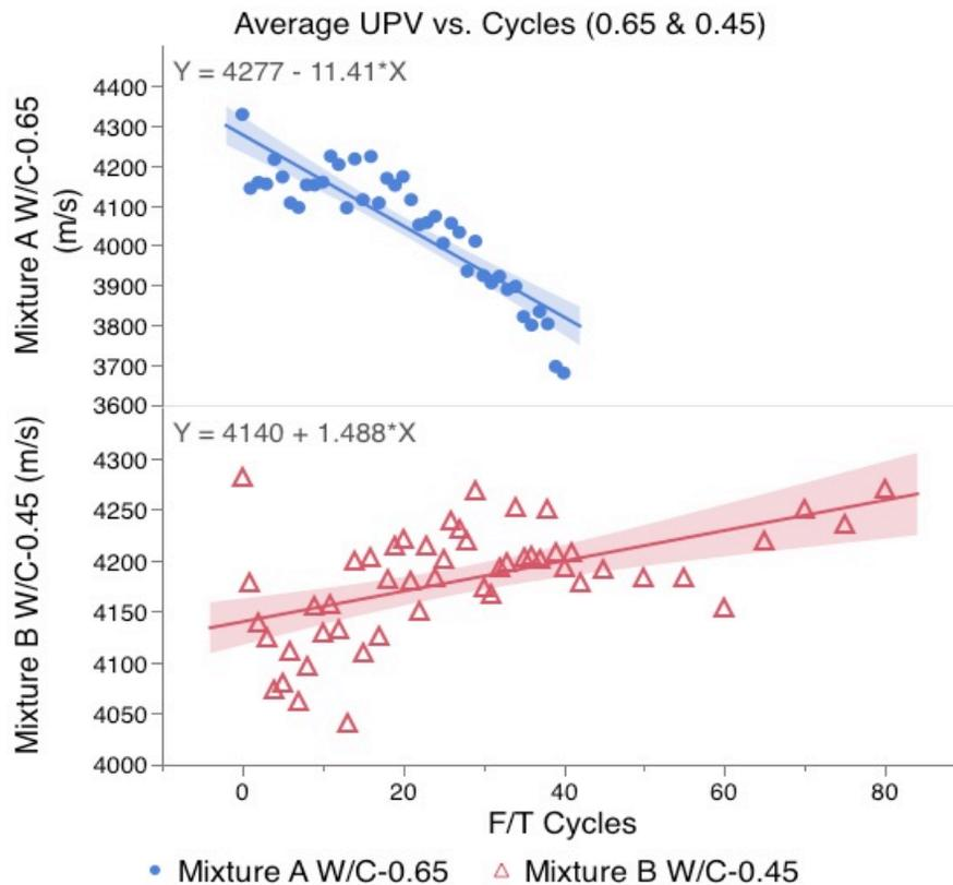
Figure 31: Average UPV vs. cycles (w/c 0.65 & w/c 0.45)
