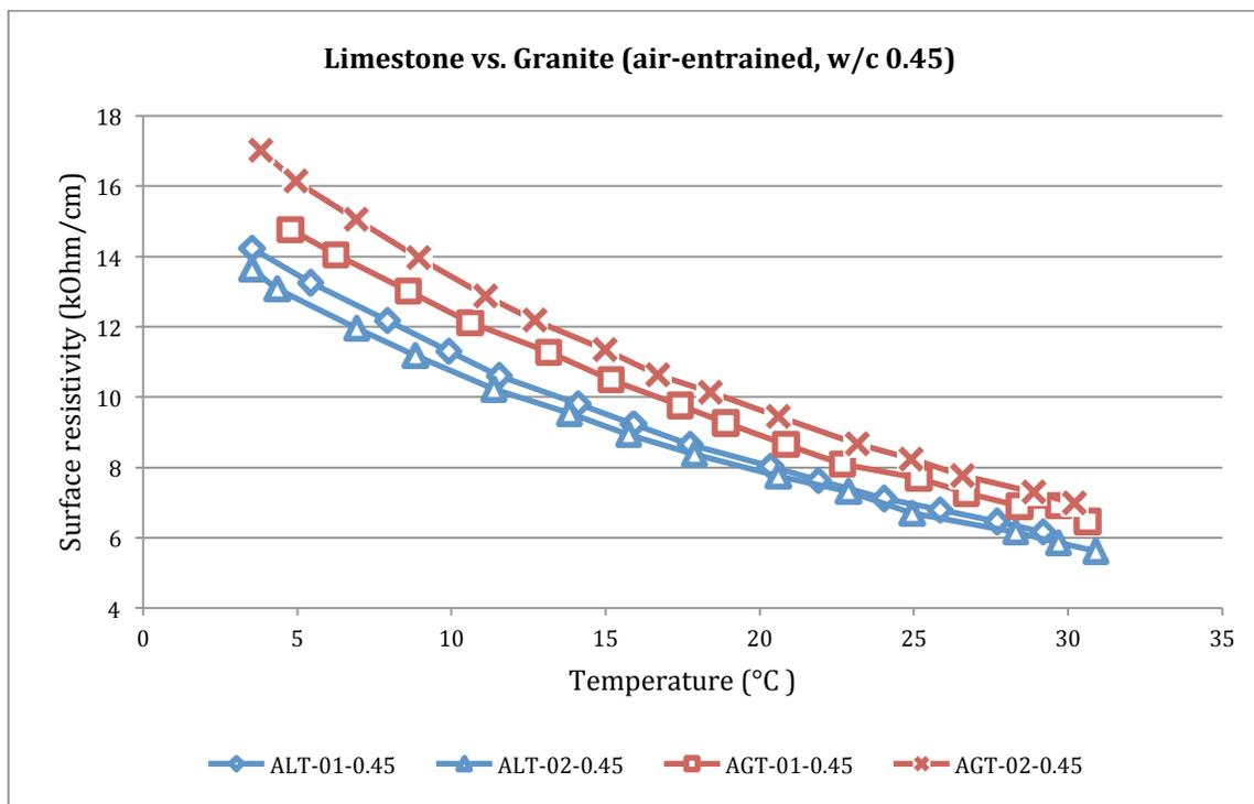
Figure 54: Limestone vs. granite (air-entrained, w/c 0.45)
