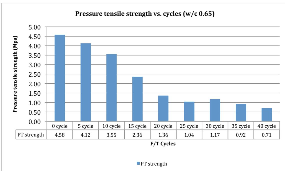
Figure 32: Pressure tensile strength vs. cycles (w/c 0.65)
