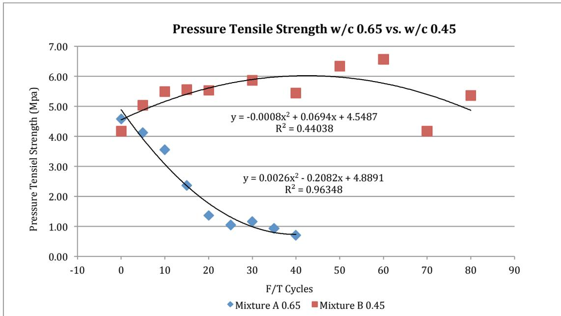
Figure 38: PT strength vs. cycles (w/c 0.65 & w/c 0.45)
