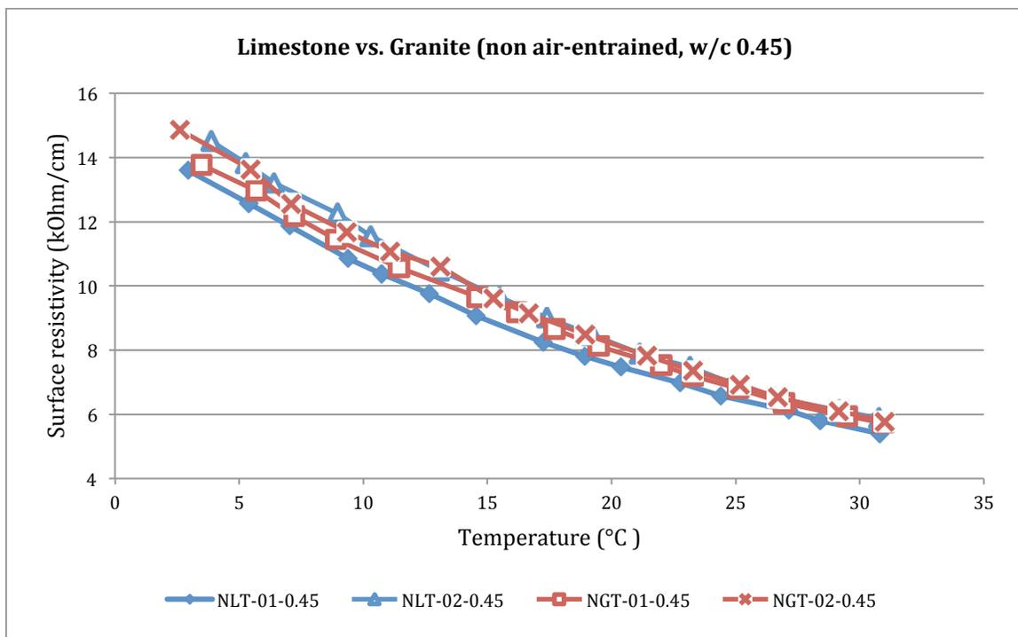
Figure 56: Limestone vs. Granite (non air-entrained, w/c 0.45)
