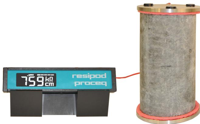
Figure 6: Proceq - Resipod bulk resistivity meter
