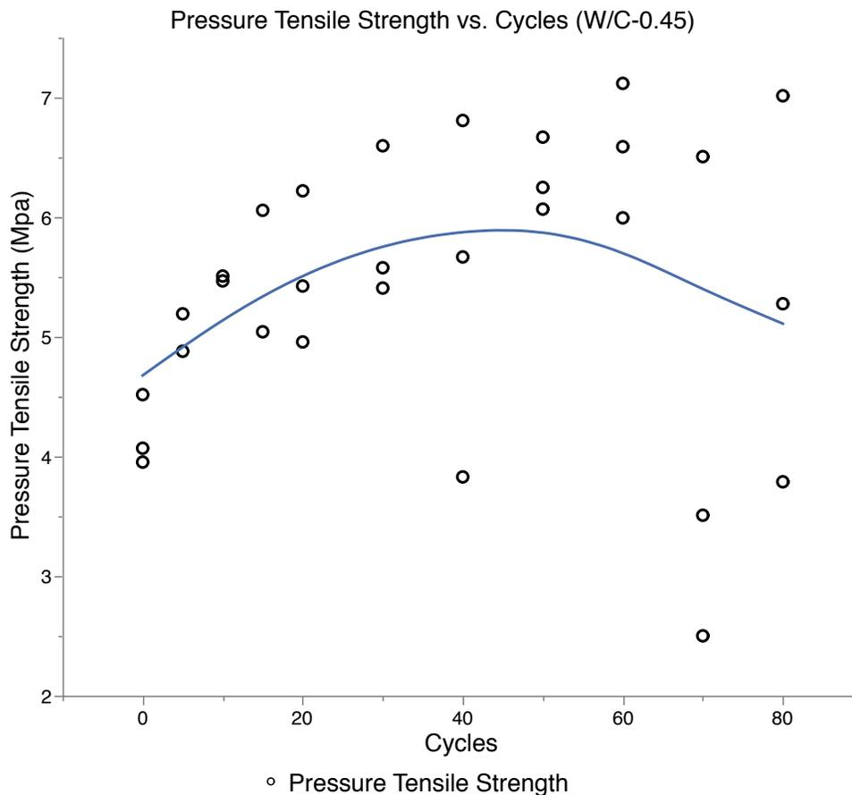
Figure 36: PT strength vs. cycles (w/c 0.45, scatter plot)
