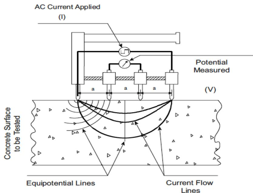
Figure 4: Four point Wenner array probe test setup
