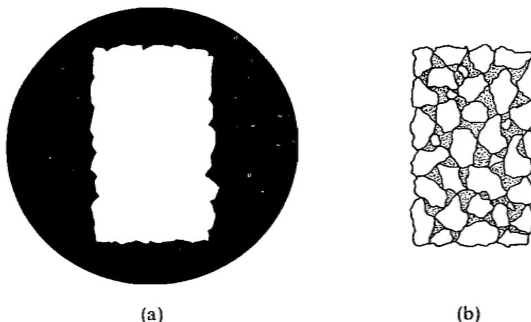
Figure 10: The diphase model (a) first order fluid and solid phase (b) second order fluid and solid phase
