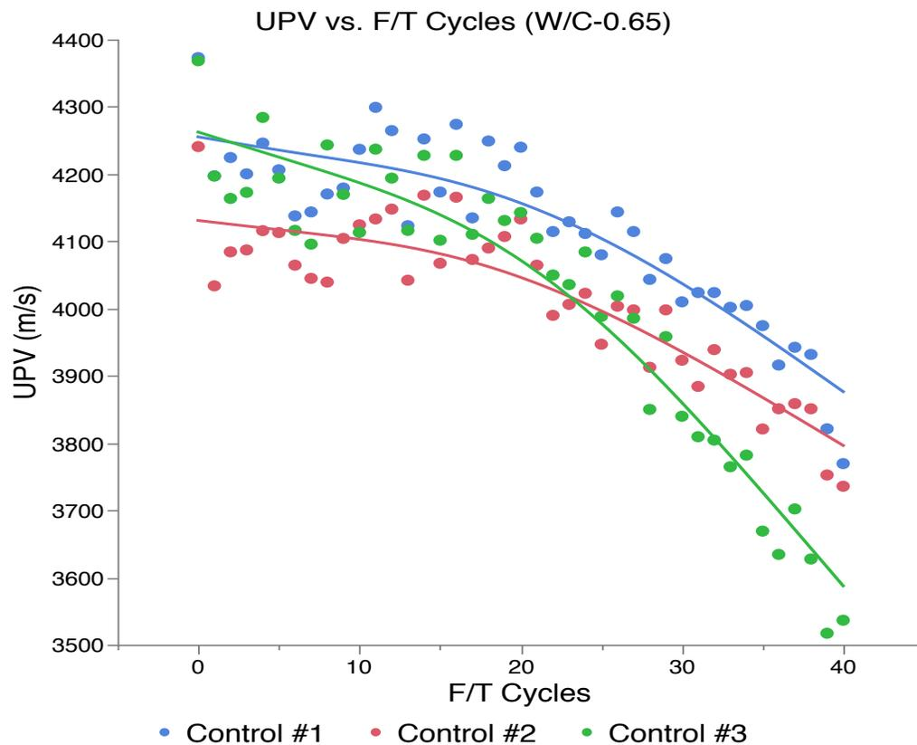
Figure 29: UPV vs. F/T cycles (w/c 0.65)
