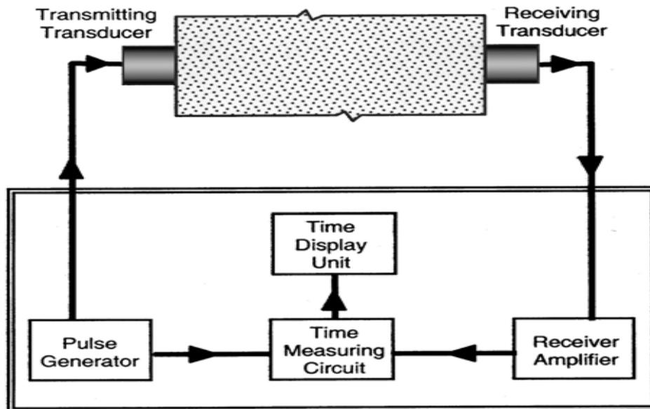
Figure 7: Schematic of pulse velocity apparatus
