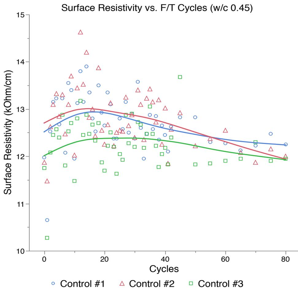
Figure 23: Surface resistivity vs. F/T cycles (w/c 0.45)
