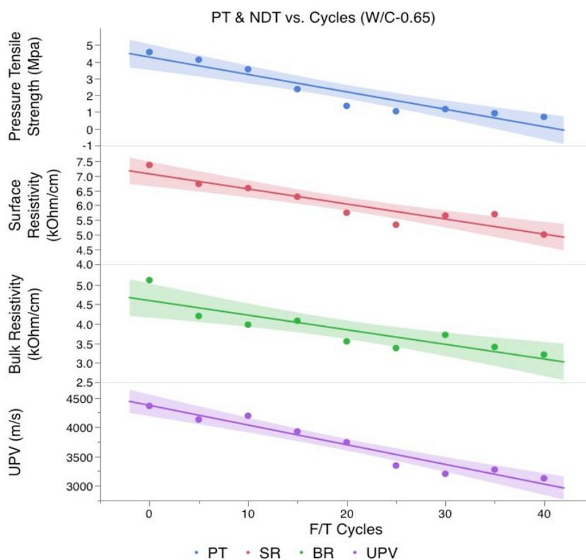
Figure 39: PT & NDT vs. cycles (w/c 0.65)
