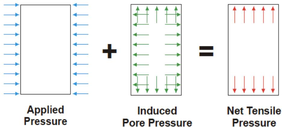
Figure 9: The mechanism of the pressure tension test
