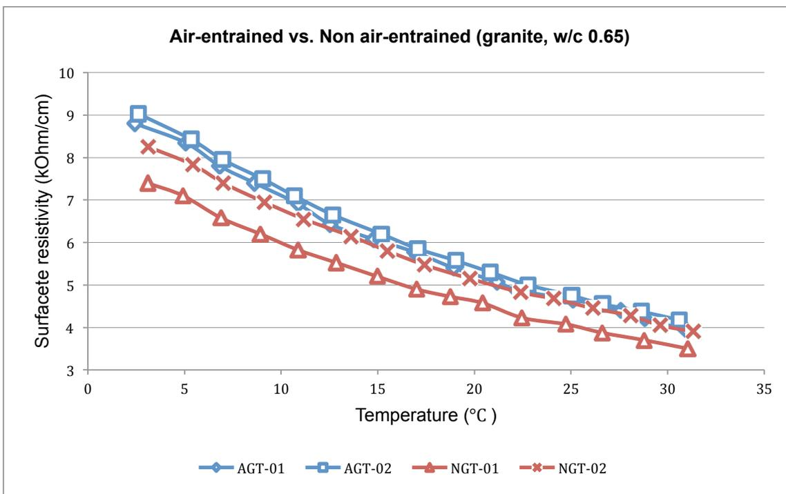
Figure 59: Air-entrained vs. non air-entrained (granite, w/c 0.65)
