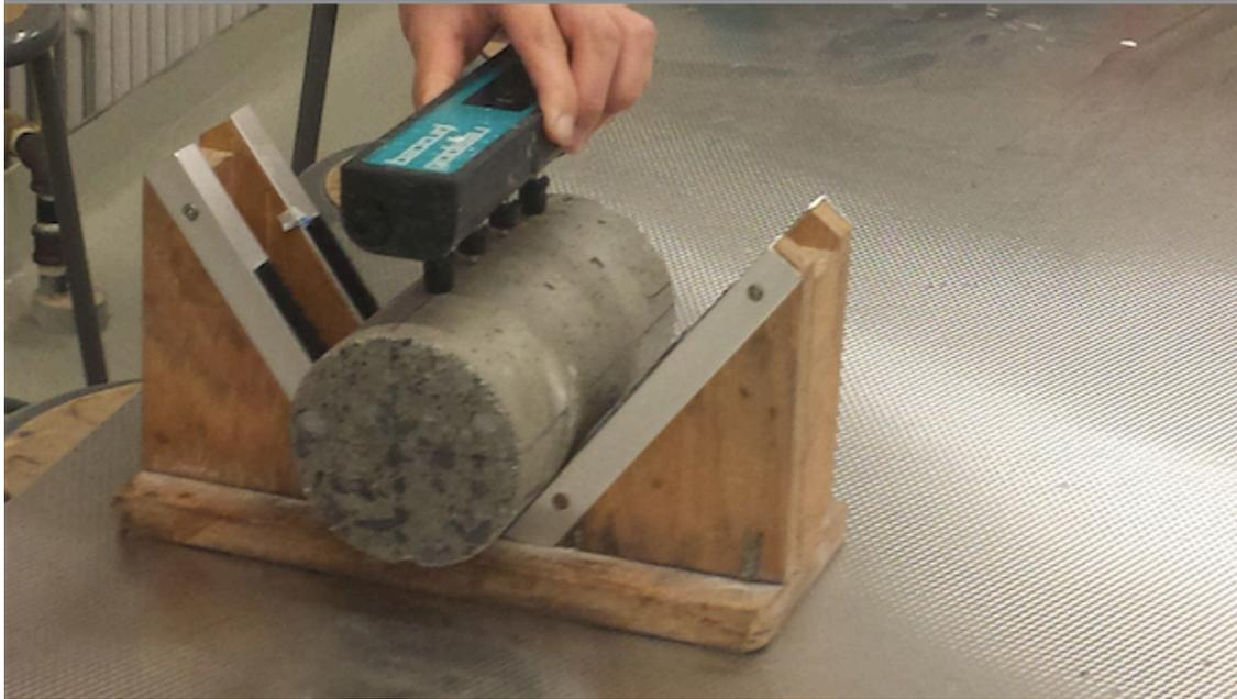
Figure 18: Testing surface resistivity using Resipod
