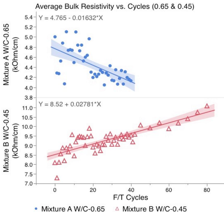
Figure 28: Average bulk resistivity vs. cycles (w/c 0.65 & w/c 0.45)
