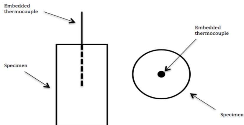
Figure 13: Schematic of specimen with thermocouple
