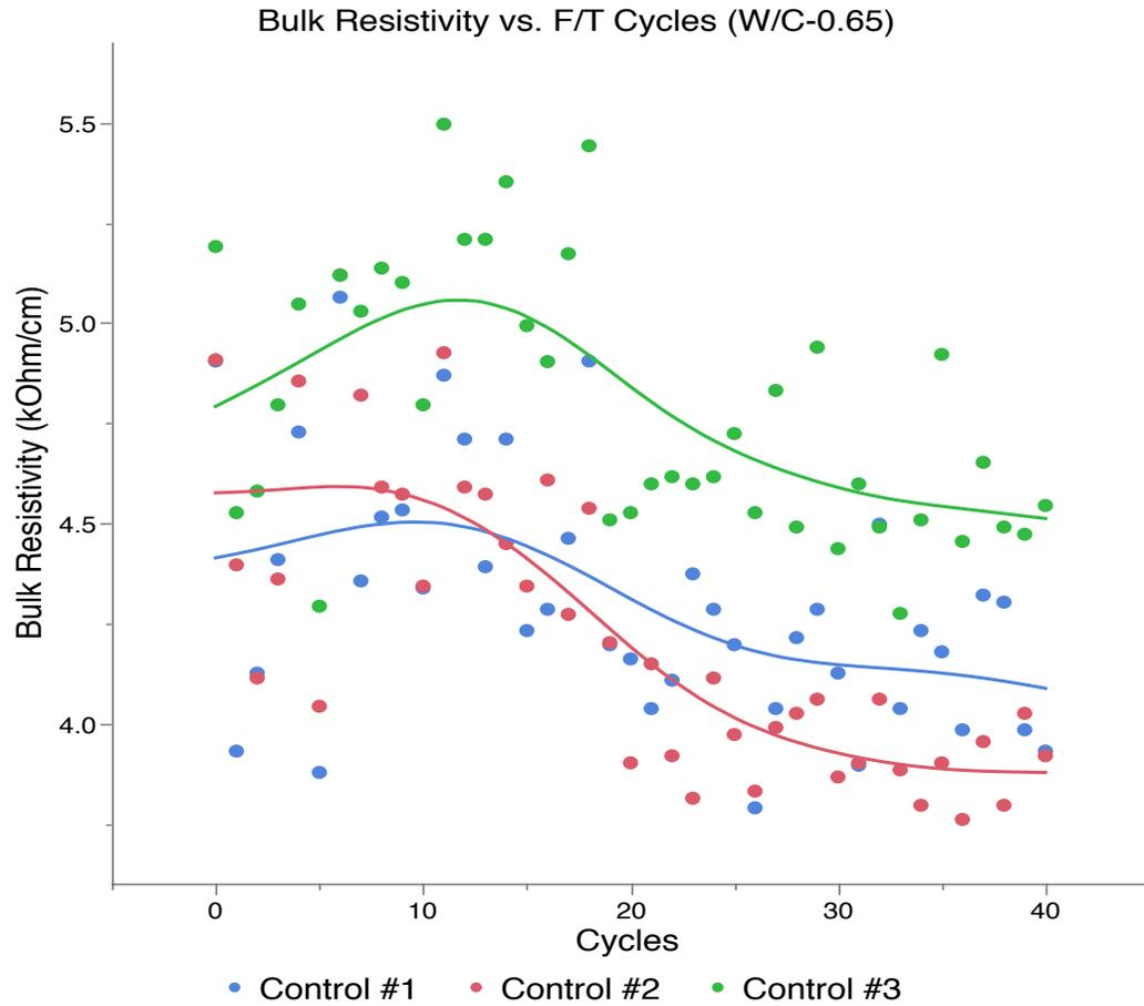
Figure 26: Bulk resistivity vs. F/T cycle (w/c 0.65)
