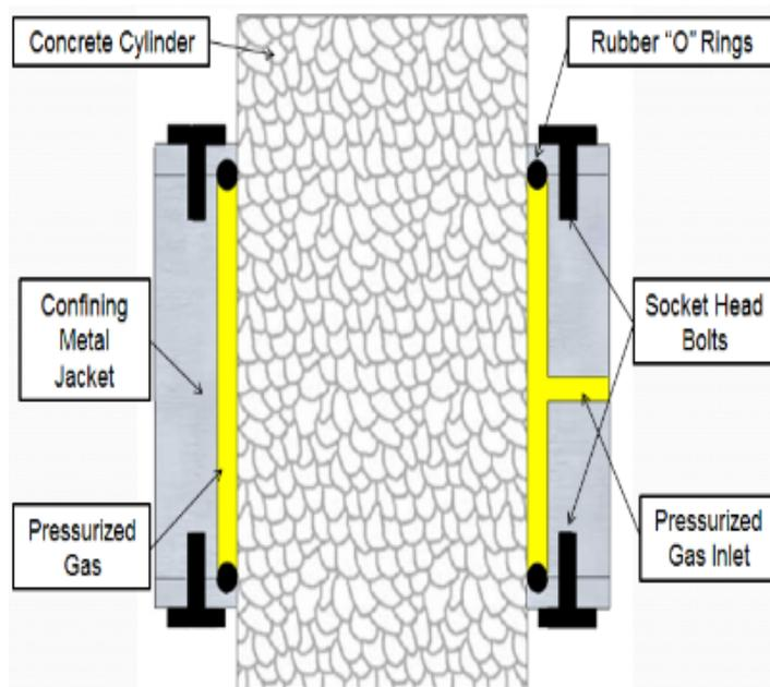
Figure 11: Schematic of pressure tension test
