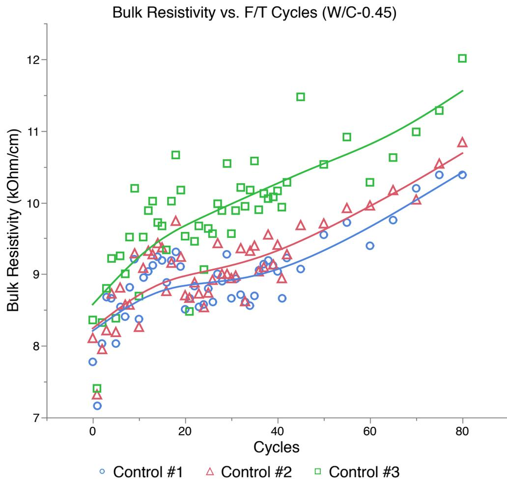
Figure 27: Bulk resistivity vs. F/T cycles (w/c 0.45)
