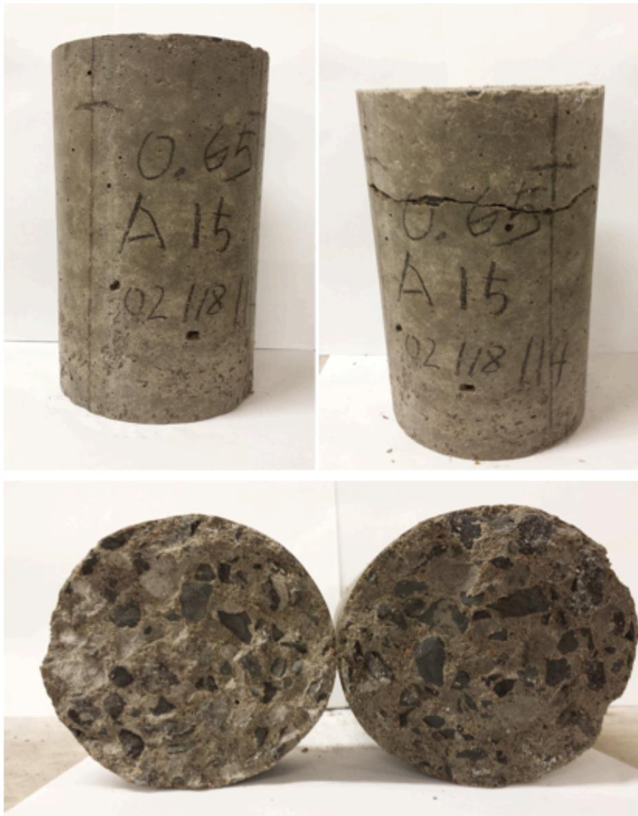
Figure 33: Specimen #15 of Mix 0.65 after 20 cycles
