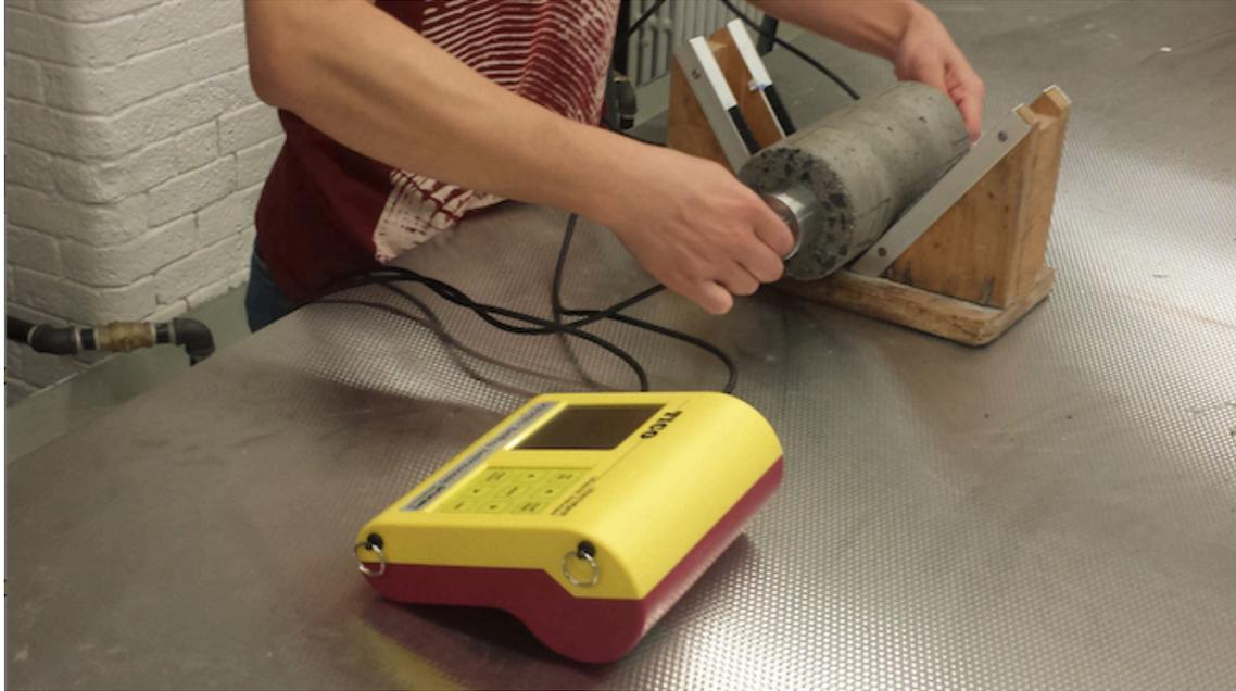
Figure 19: Operation of ultrasonic pulse velocity test
