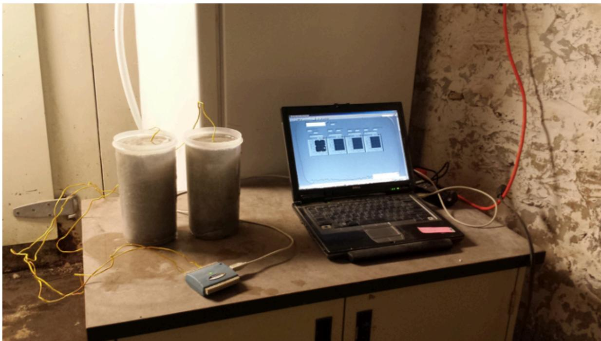
Figure 14: Monitoring temperature using thermocouples
