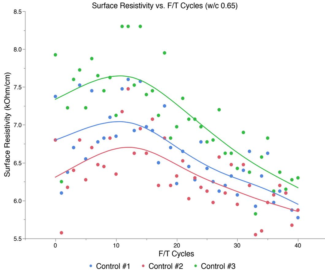
Figure 21: Relationship between surface resistivity and F/T cycles
