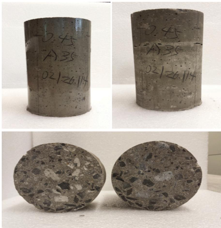
Figure 37: Specimen #35 of Mix 0.65 after 80 cycles
