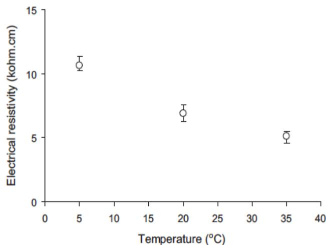
Figure 47: Effect of temperature on electrical resistivity
