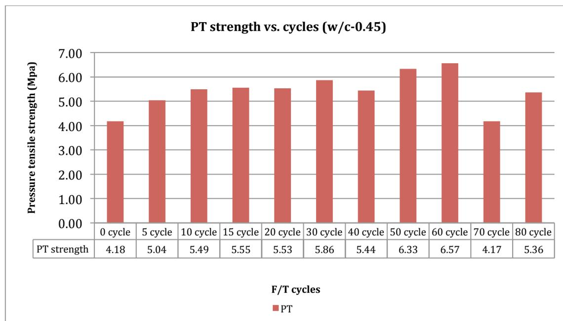
Figure 35: PT strength vs. cycles (w/c 0.45)
