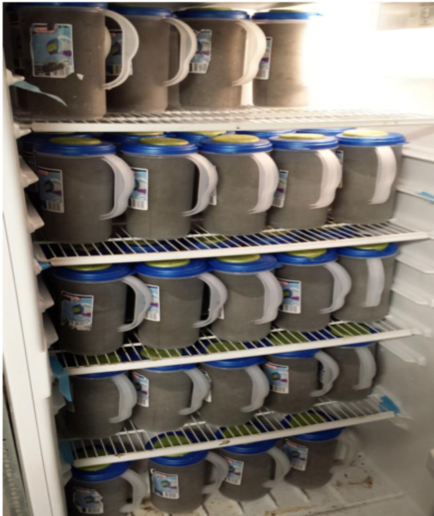
Figure 15: Concrete specimens undergoing freezing process
