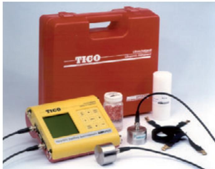
Figure 8: Proceq - TICO ultrasonic pulse velocity
