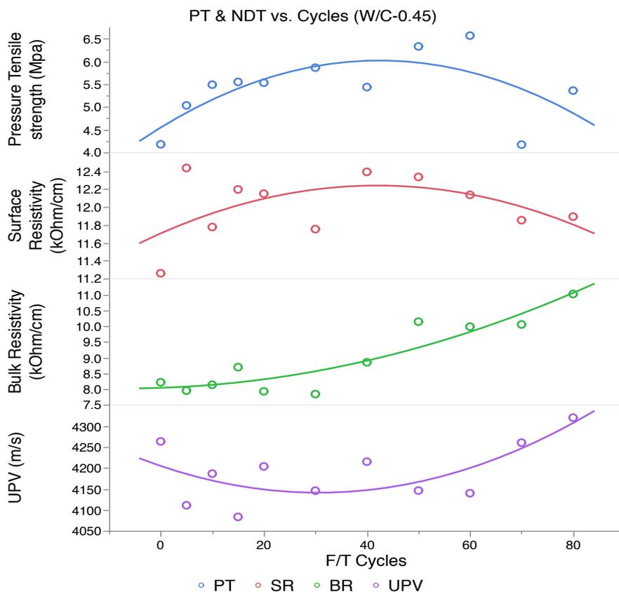
Figure 40: PT & NDT vs. cycle (w/c 0.45)
