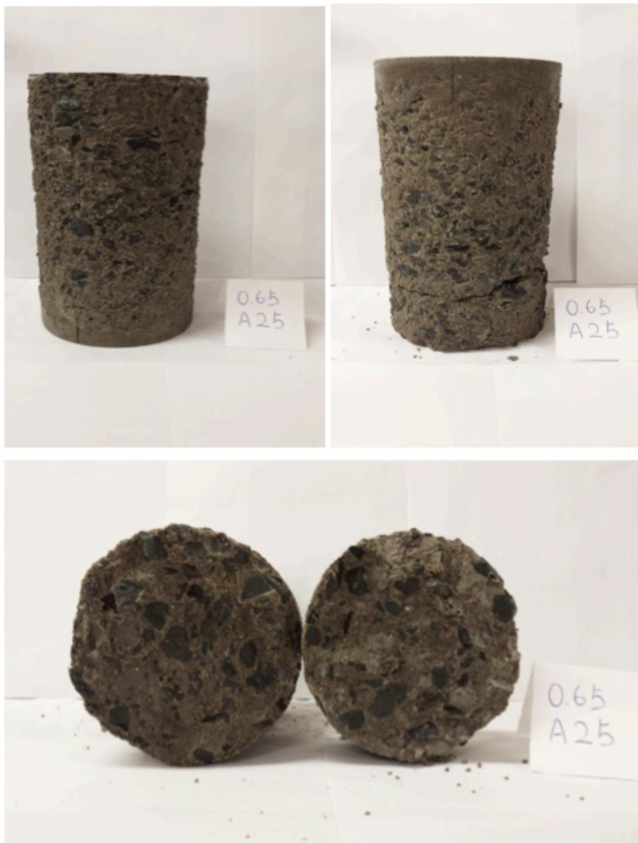
Figure 34: Specimen #25 of Mix 0.65 after 40 cycles
