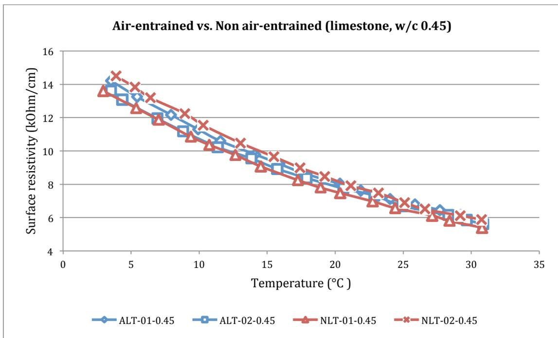
Figure 58: Air-entrained vs. non air-entrained (limestone, w/c 0.45)
