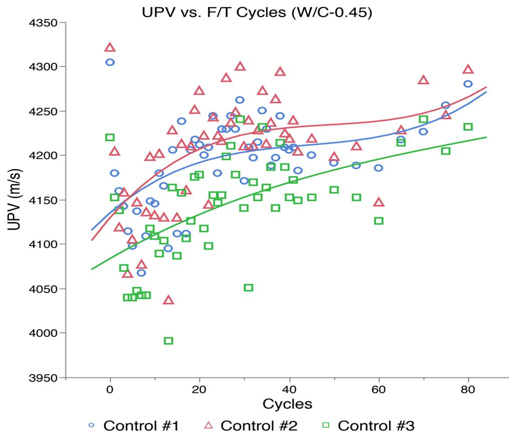
Figure 30: UPV vs. F/T cycles (w/c -0.45)
