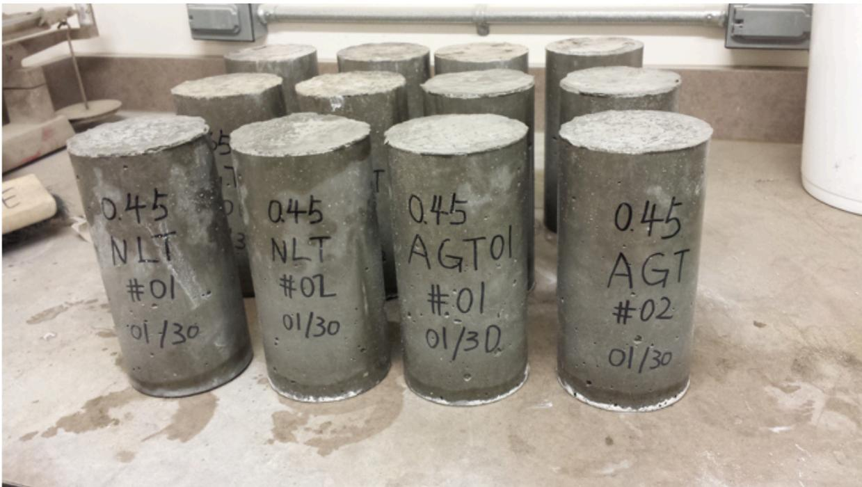
Figure 48: Marked specimens after demoulding
