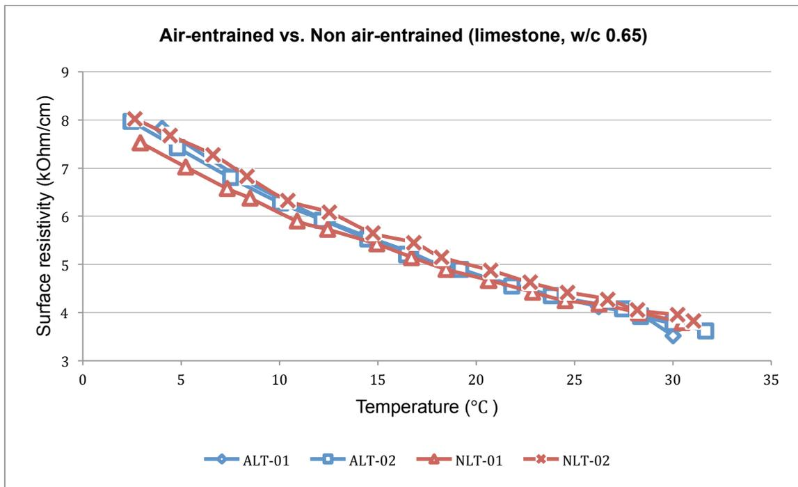
Figure 57: Air-entrained vs. non air-entrained (limestone, w/c 0.65)
