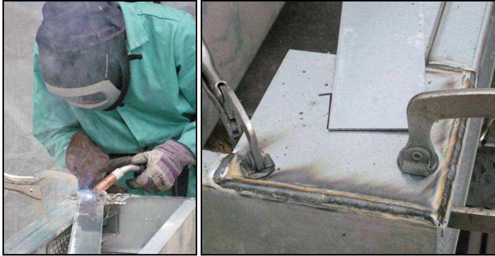
Figure 2.6: Welding process and partially finished weld pattern on a medium wall
