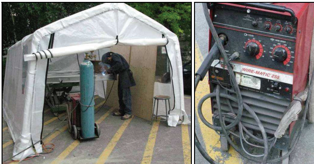
Figure 2.5: Welding setup and Lincoln Electric GMAW welder
