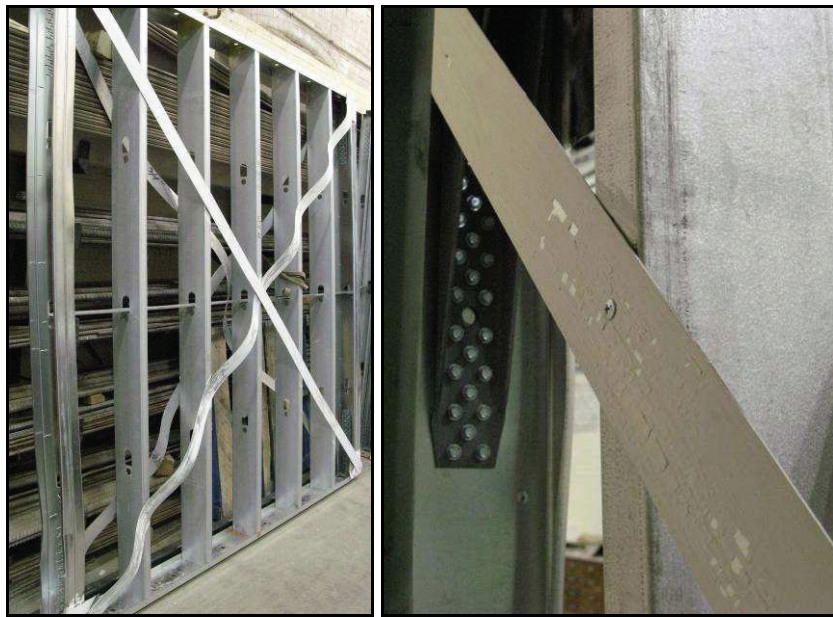
Figure 2.23: Medium walls showing brace yielding
