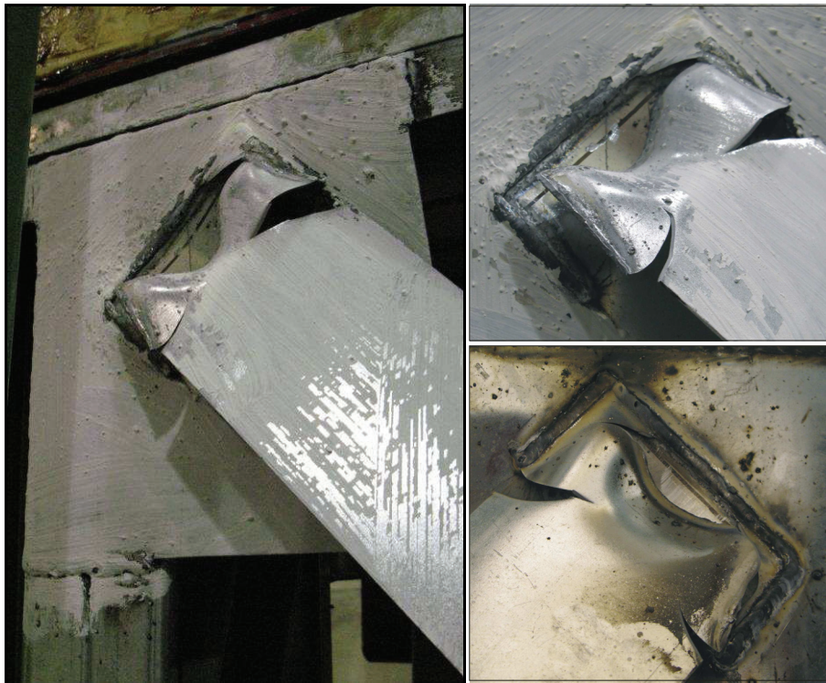
Figure 2.13: Connection failure of preliminary test 21A-M
