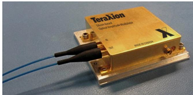
FIGURE 4–9: Picture of the fully packaged SiP modulator.
