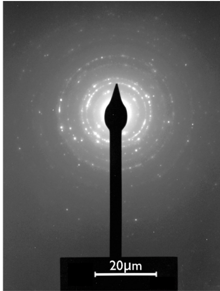
Figure 16: Selected area diffraction (SAD) of an as-sprayed HVOF CoNiCrAlY coating
