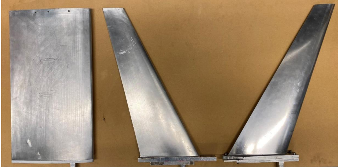
Figure 3-2 Three wing models tested. (left) rectangular wing, (middle) backward swept wing, and (right) forward swept wing.
