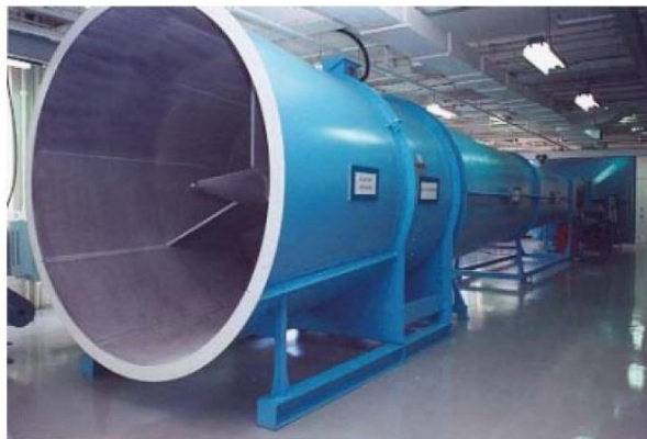
Figure 3-1 Schematic of J.A. Bombardier wind tunnel. (a) schematic diagram, (b) wind tunnel inlet and (c) outlet. (Pereira 2011)
