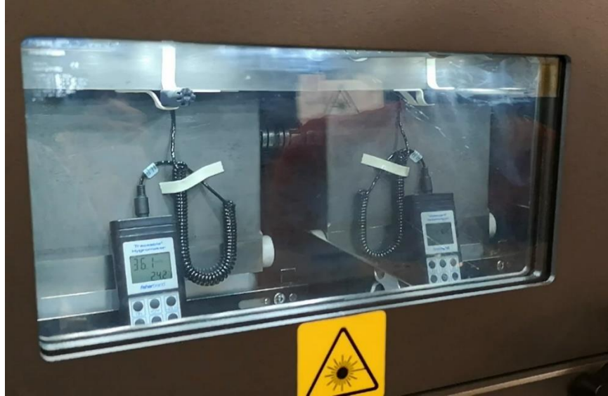
Figure 3.4. External view of the mounted probe hygrometer displaying the RH inside the build chamber of a Renishaw AM 250 LPBF unit.
