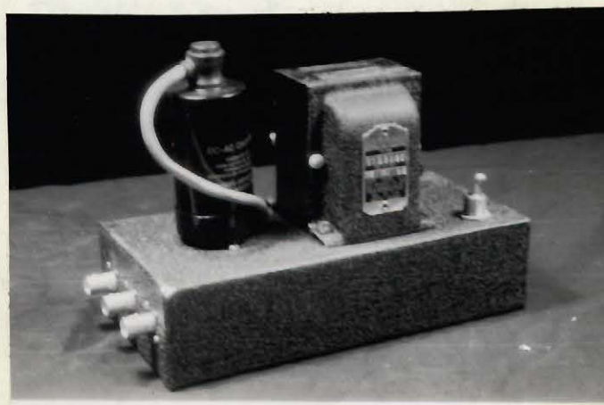
Figure 6.3 60 cycle Switching Relay , showing BNC connectors.
