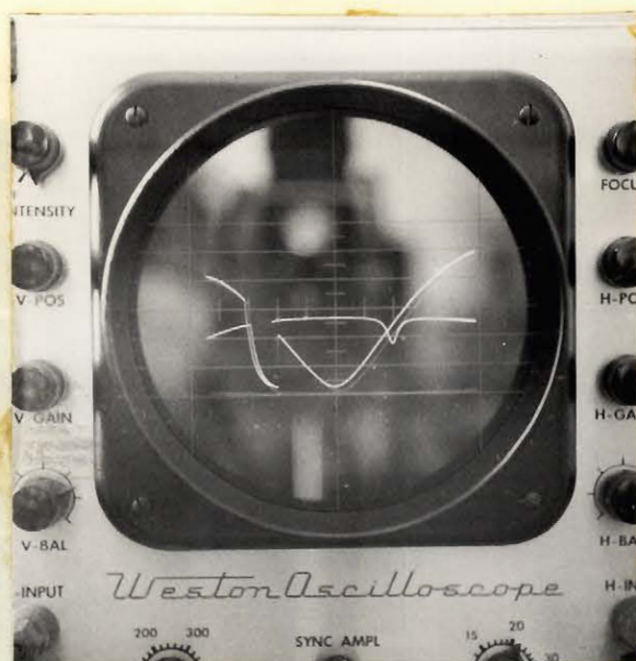
Figure 5.2 A typical oscillographic display. The horizontal trace is the incident power, the small dip in it the wavemeter indication. The wider response curve is the reflected power.
