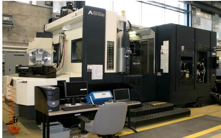
Figure 4-1 Makino A88ε machining center used for drilling tests
