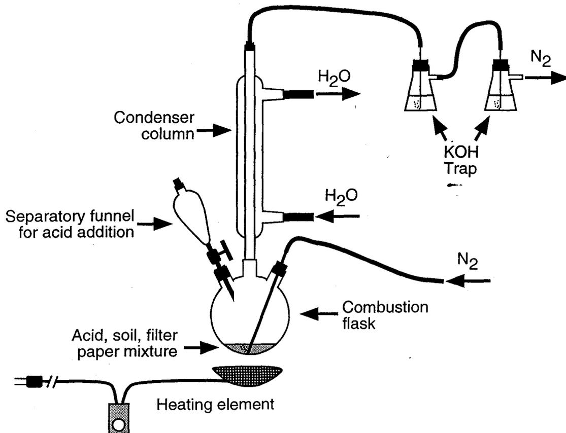
Figure 6.1. Schematic of the soil combustion apparatus.
