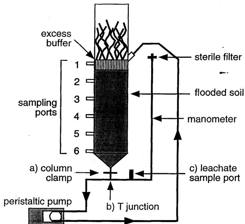
Figure 5.1. Schematic of flooded soil columns. Buffer was circulated at 2 mL/minute in the direction indicated. The portion of the columns containing the flooded soil was covered with aluminum foil.
