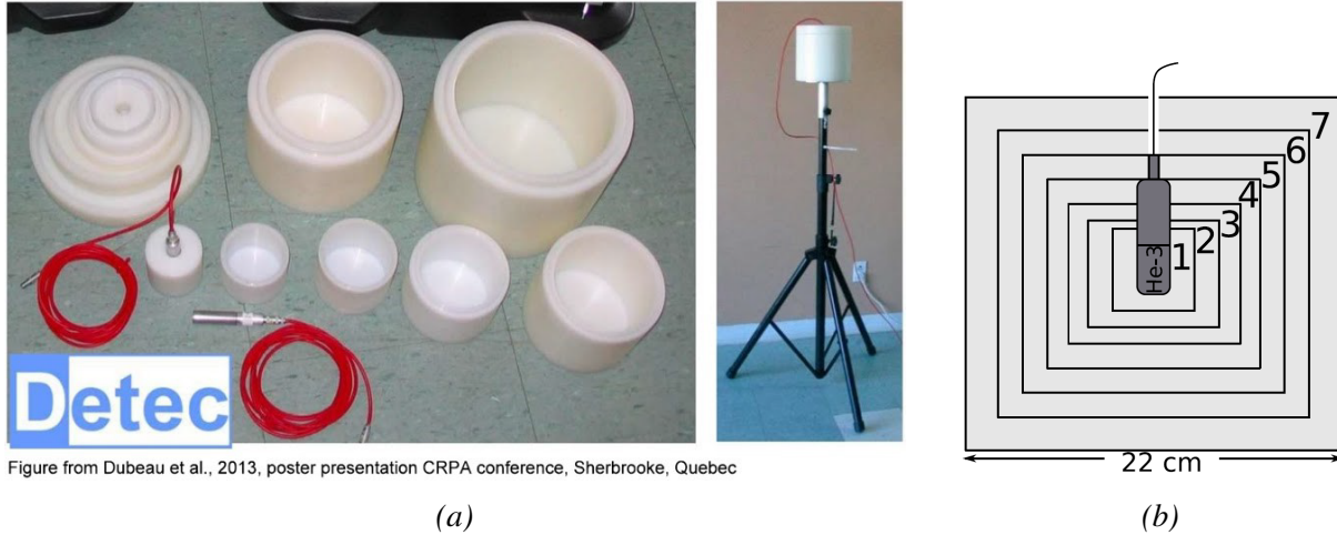
Figure 1.3 – The Nested Neutron Spectrometer (NNS). (a) Photographs of the ^3\text{He} chamber, concentric moderator shells, and final assembly mounted on a tripod. (b) A schematic cross section of the NNS showing the ^3\text{He} chamber at the geometrical center [21].
