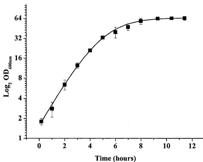
Figure 5.2 Growth in fed-batch LPI culture inoculated with 10 mM monobasic ammonium phosphate and 12 ml/hr linear feed rate. No induction was observable.
