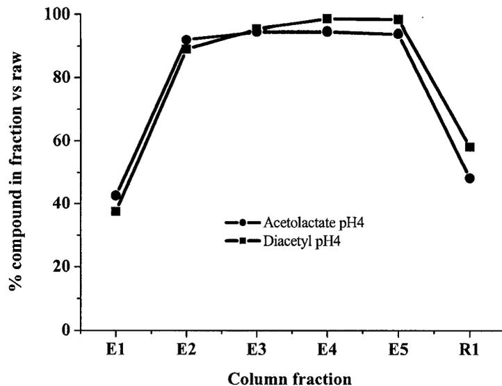
Figure 7.6. Analysis of  $\alpha$ -acetolactate and diacetyl retention by a Sepak C-18 mini column at pH 4.0. 1ml fractions were eluted (E) prior to column rinsing (R).
