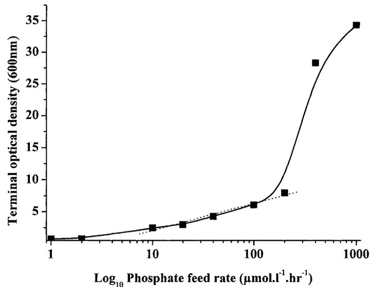
Figure 5.6 Analysis of final cell yield versus phosphate feed rate. A dramatic change in yield is observed for feed rates higher than 200  $\mu\text{mol/l/hr}$ .
