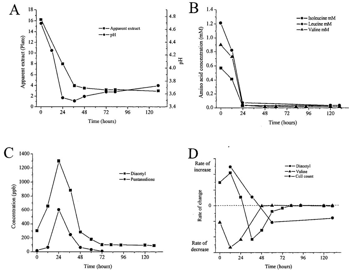
Figure 6.2. Ale yeast fermentation profile at 20 °C. (A) Apparent extract and pH profiles, (B) isoleucine, leucine and valine profiles, (C) diacetyl and pentanedione profiles and (D) rates of change in valine consumption, diacetyl production and cell concentration.
