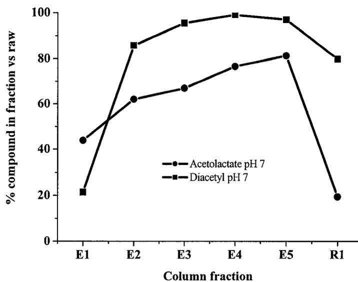
Figure 7.7. Analysis of  $\alpha$ -acetolactate and diacetyl retention by a Sepak C-18 mini column at pH 7.0. 1ml fractions were eluted (E) prior to column rinsing (R).
