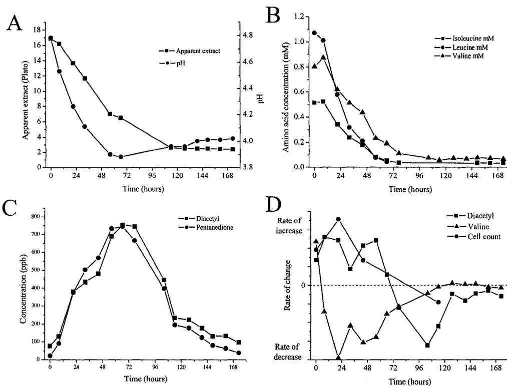
Figure 6.3. Lager yeast fermentation profile at 14 °C. (A) Apparent extract and pH profiles, (B) isoleucine, leucine and valine profiles, (C) diacetyl and pentanedione profiles and (D) rates of change in valine consumption, diacetyl production and cell concentration.
