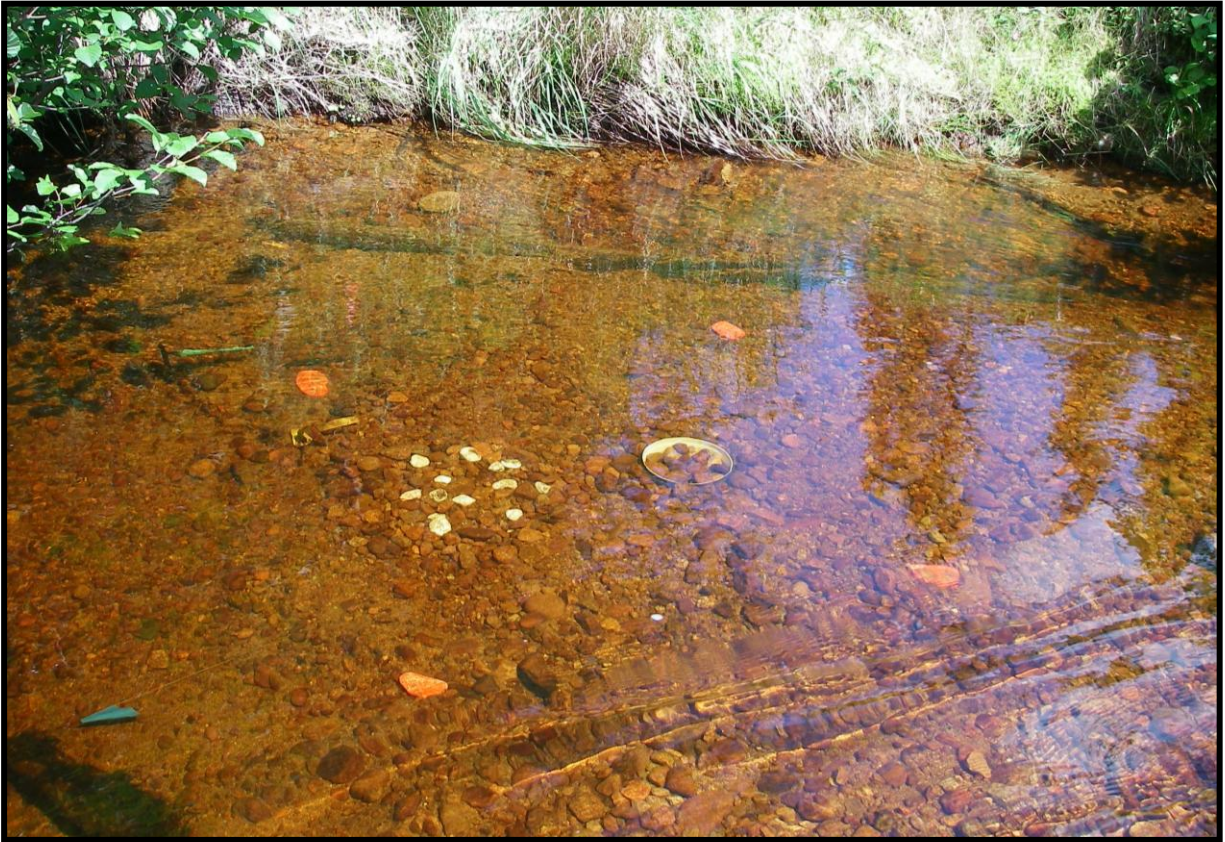
Figure 5.1. Photograph showing typical experimental redd installation. Photo taken immediately following installation. Water flow is from left to right. White marker gravels ( D_{90} caliber) denote location of the experimental redd. Sediment collection bucket is located approximately 50 cm downstream.
