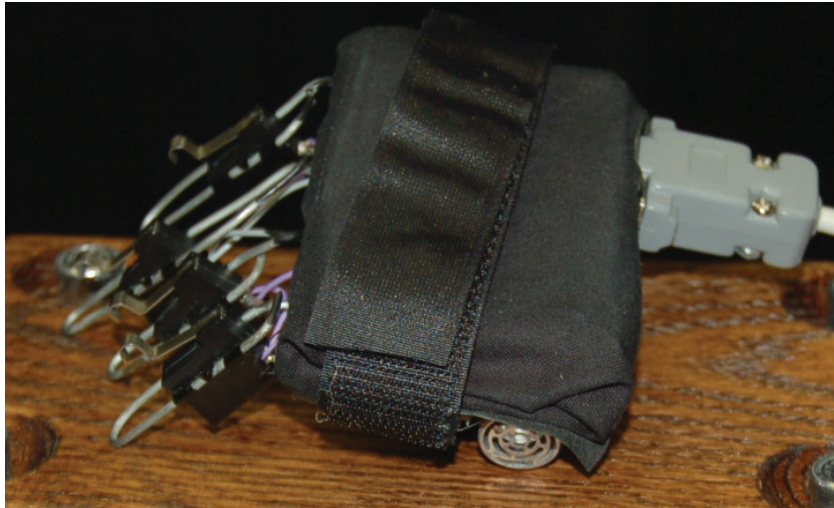
Figure 7.4: One of the T-Box hand pieces, showing the ultrasound transmitter and the finger switches.
