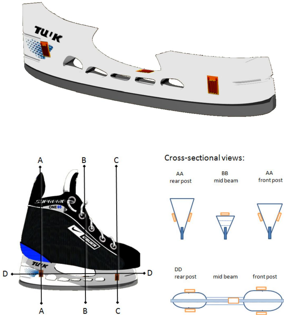
Figure 13 – Representation of instrumented skate blade holder (top), and cross-sectional views of gauge locations (bottom). Gauges AML and PML are oriented vertically along each post, while gauge V is oriented longitudinally along the beam element of the blade holder.
