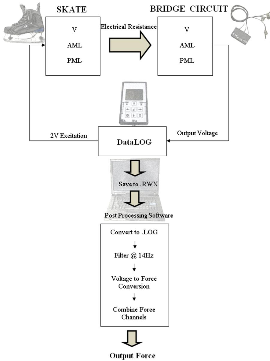
Figure 15 – Data acquisition and processing sequence.
