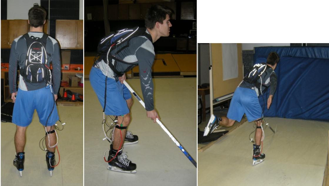
Figure 32 – Skater set-up as viewed from (1) back, (2) side, and (3) during push-off.
