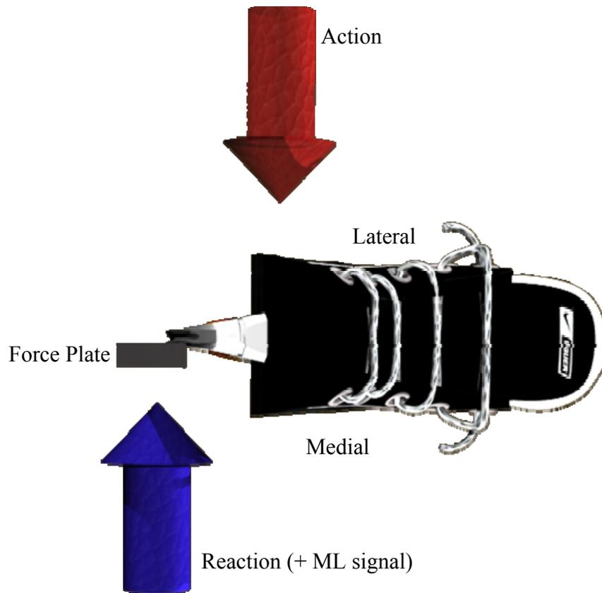
**Figure 17 – Medial validation viewed from front. The red arrow represents uniform loading, while the blue arrow represents the reaction force produced by the force plate.**
