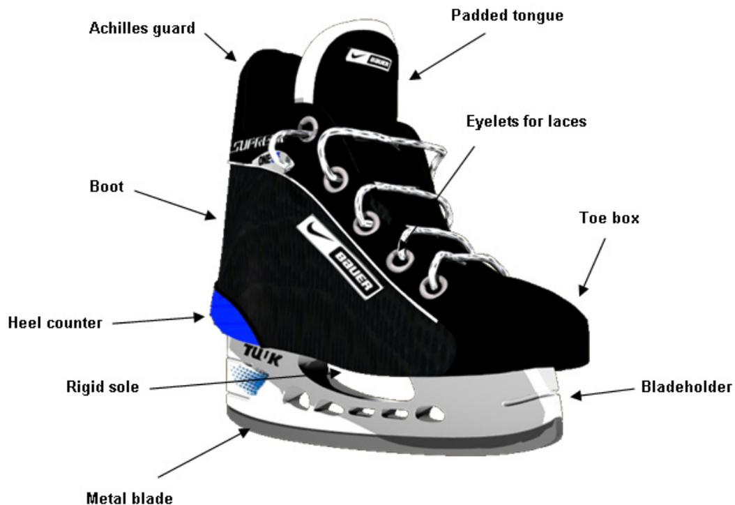
Figure 8 – Structural components of a modern hockey skate (adapted from Pearsall and Turcotte, 2007).
