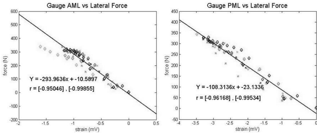
Figure 20 – (1) Gauge AML versus lateral force, and (2) gauge PML versus lateral force.
