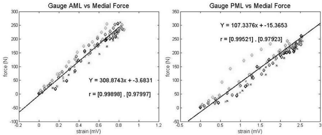
Figure 19 – (1) Gauge AML versus medial force, and (2) gauge PML versus medial force.
