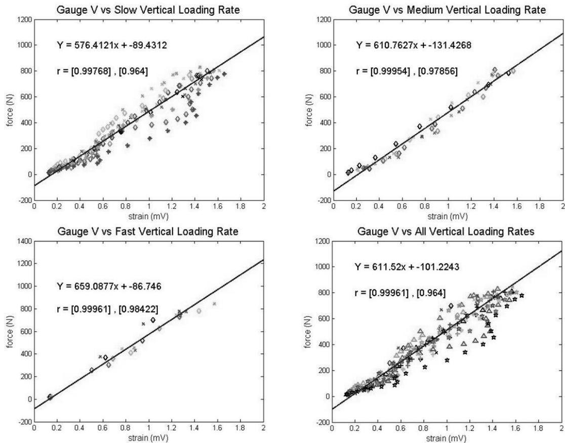
**Figure 18 – (1) Gauge V versus slow vertical loading rate, (2) Gauge V versus medium vertical loading rate, (3) Gauge V versus fast vertical loading rate, and (4) Gauge V versus all vertical loading rates.**
