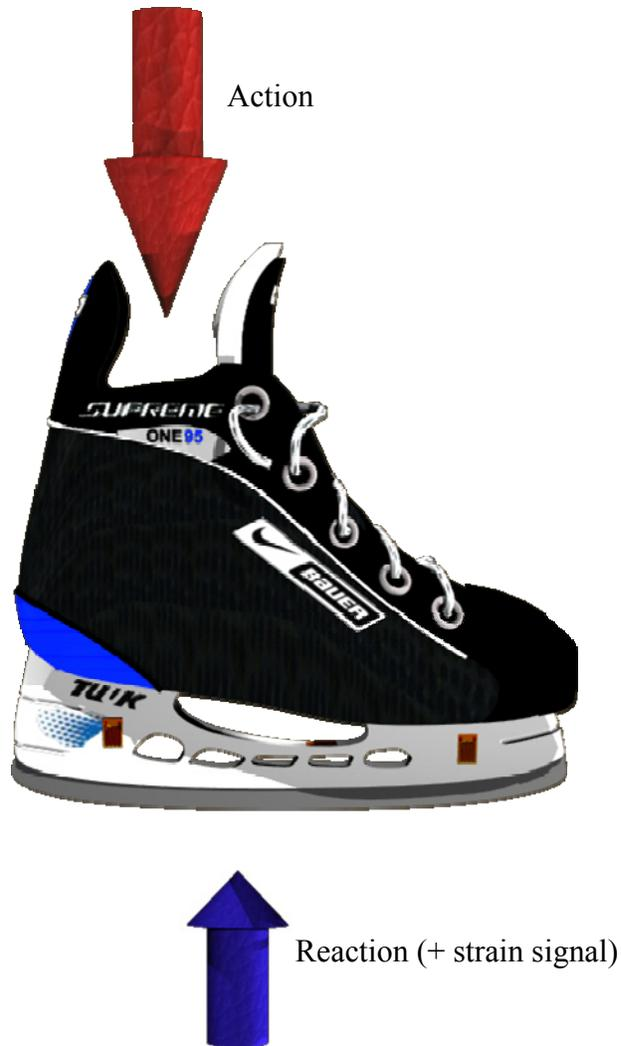
**Figure 16 – Vertical validation viewed from side. The red arrow represents uniform loading throughout the skate, while the blue arrow represents the reaction strain signal.**
