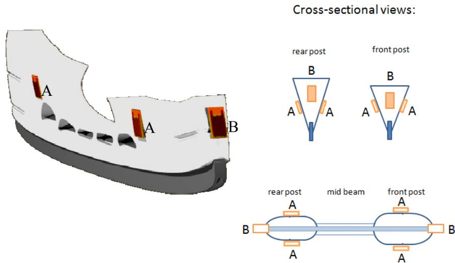
**Figure 6 – Depiction of gauge placement used by Lamontagne et al. (1983) on plastic blade holder (adapted from Lamontagne et al., 1983). A denotes gauges used to determine compressive (normal) forces, B denotes gauges used to determine flexile (medial-lateral) forces.**
