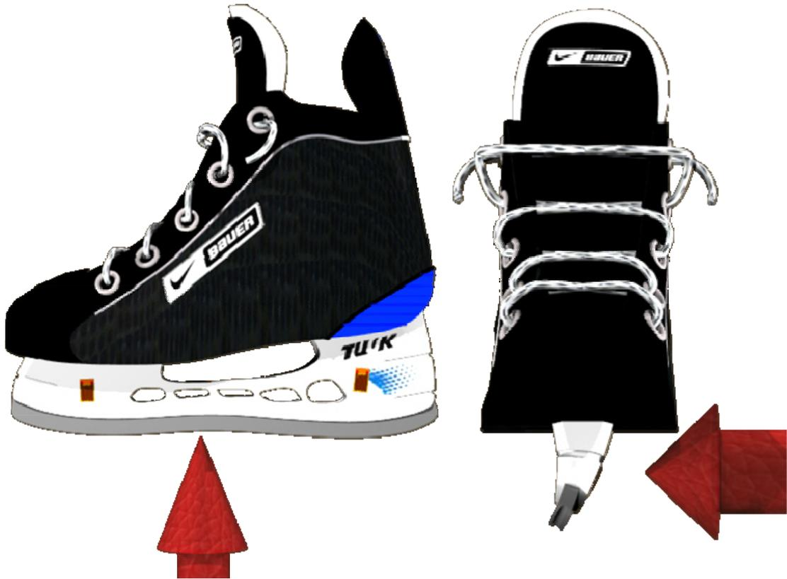
Figure 14 – Exaggeration of deformation caused by vertical loading (left) and deformation caused by lateral loading (right).
