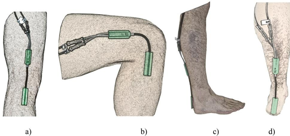
Figure 26 – Placement of the Elgons about the subject's knee(a, extended, b, flexed) and ankle (c,side view, d, rear view)
