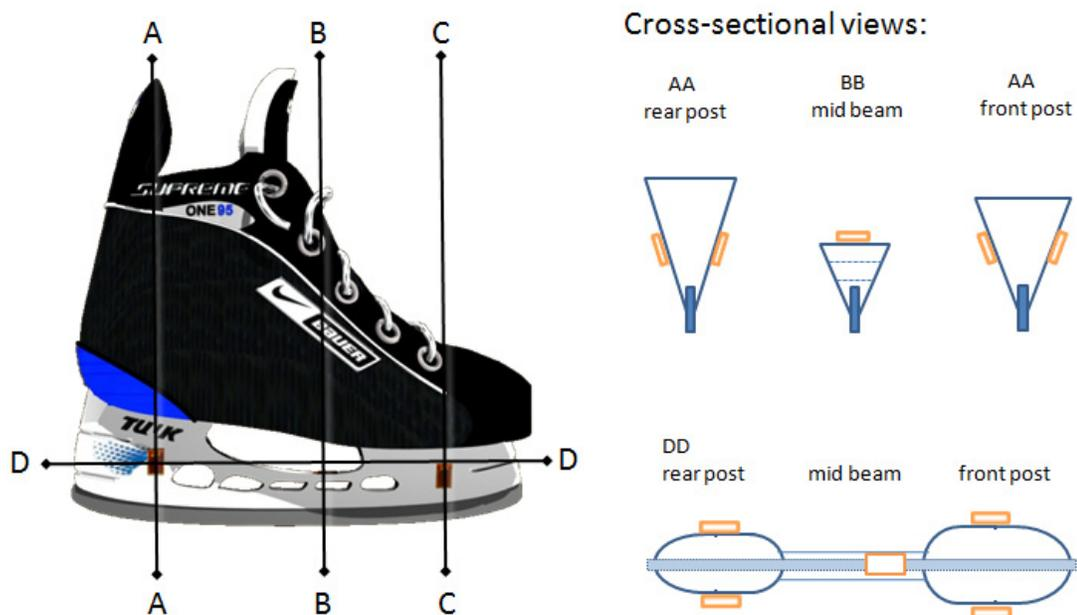
Figure 25 – Representation of cross-sectional views of gauge locations
