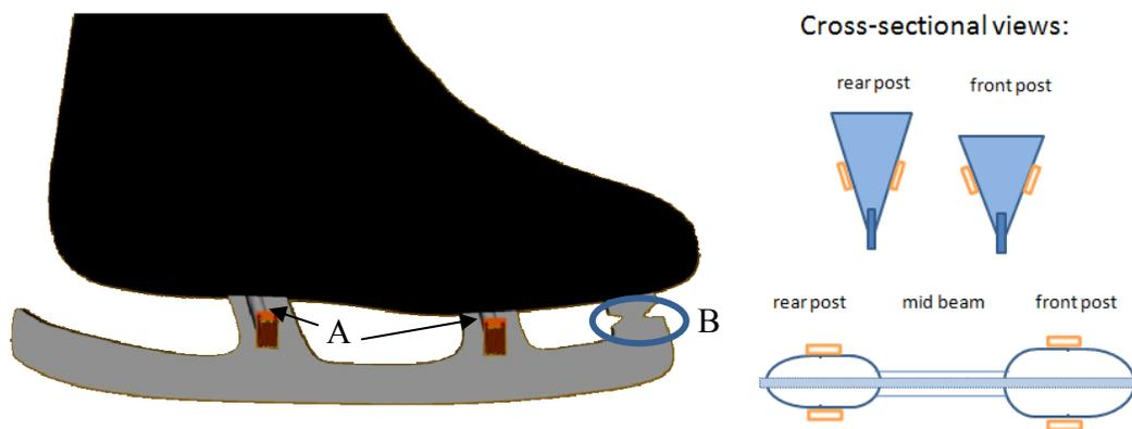
**Figure 7 – Depiction of gauge placement used by Lamontagne et al. (1983) on metal bladeholder (adapted from Lamontagne et al., 1983).**
