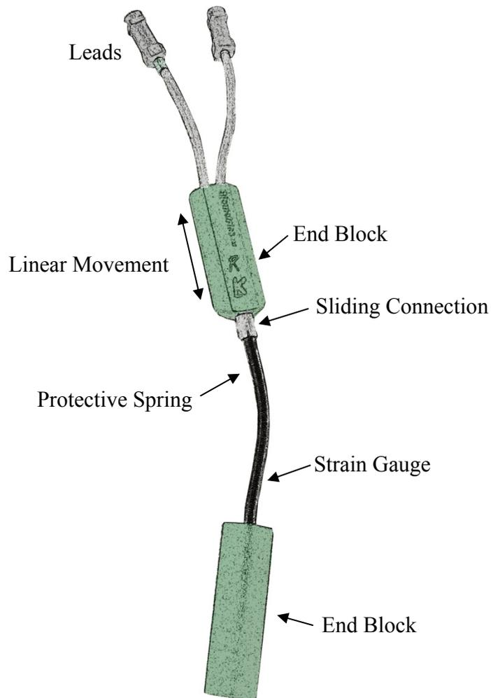
**Figure 10 – Electrogoniometer (adapted from Goniometer and Torsinometer operating manual, 2002).**
