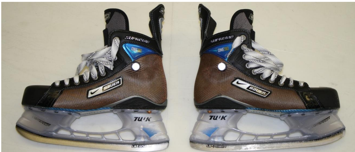
Figure 10: Pair of skates fitted with passive reflective markers on the lateral malleoli.
