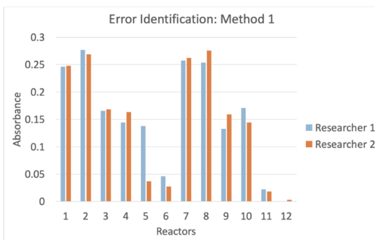
Figure B.1: P -measurement using the Molybdovanadate (yellow method) was carried out by another independent researcher. The wavelength of the supernatant samples was spectrophotometrically measured at 470 nm. The absorbance data from both researchers was not significantly different ( t(22)=2.07 , p>0.05 ).
