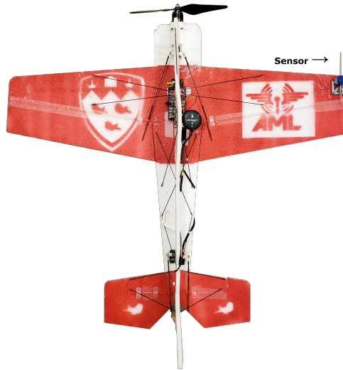
Figure 4.20: Sample of wind rejection setup showing airspeed sensor location
