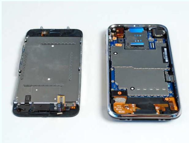
**Fig 4.9** An example of a metallic shielding box in a mobile handset: the interior of the Apple iPhone 3GS features a metallic shielding box to house the circuit boards. Image source: [70]
