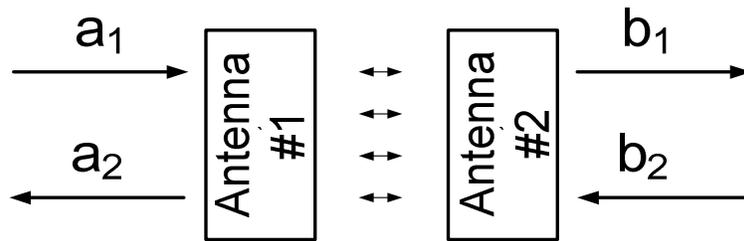
Fig. 3.2: The Definition of Scattering Parameters for a two Antenna System.
