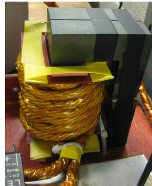
(b)  $L_{OUT}$ : custom-made ferrite-core inductor made with Litz wire.
