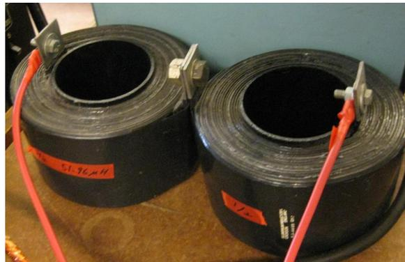
(c)  $L_2$ : air-core inductor made with aluminum.
