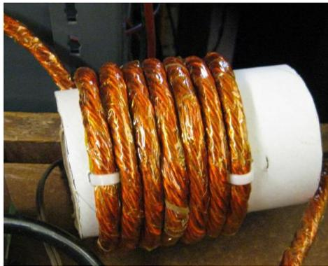
(a)  $L_1$ : custom-made air-core inductor made with Litz wire.
