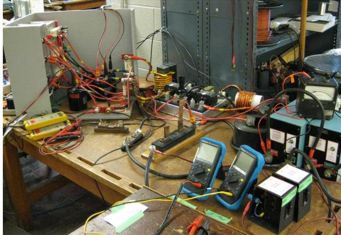
Figure 7.2: Experimental setup for 5kW prototype converter with two stages and two capacitors per stage.
