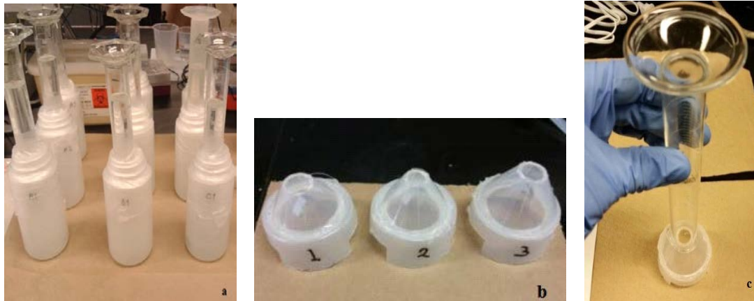
Fig. 4.2.2.1.1: (a) Immersion test set up, (b) the funnels used for attaching the alloy samples, (c) assembly of the funnel and the cylinders.
