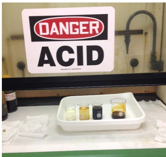
Fig. 4.2.2.3.1: The removal of corrosion layer on the samples using chromic acid ((180 g CrO 3 /dm 3 )).
