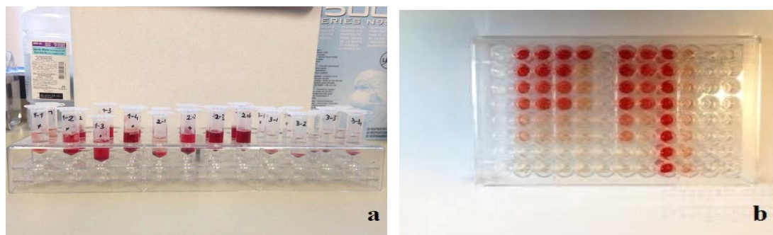
Fig. 4.4.1.1: (a) The blood samples mixed with Mg alloy particles after incubation and centrifugation, (b) blood samples transferred to a reading plate for spectroscopy.
