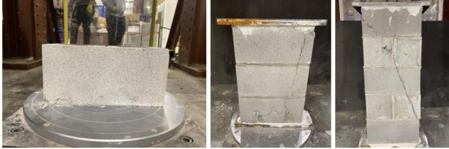
Fig. 5. Block and masonry compression tests: concrete blocks, triplets, prisms
