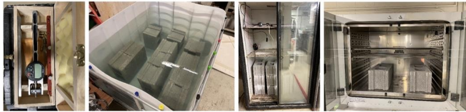
Fig. 3. DEMEC strain gauge system, immersion tank, refrigerator, drying oven
