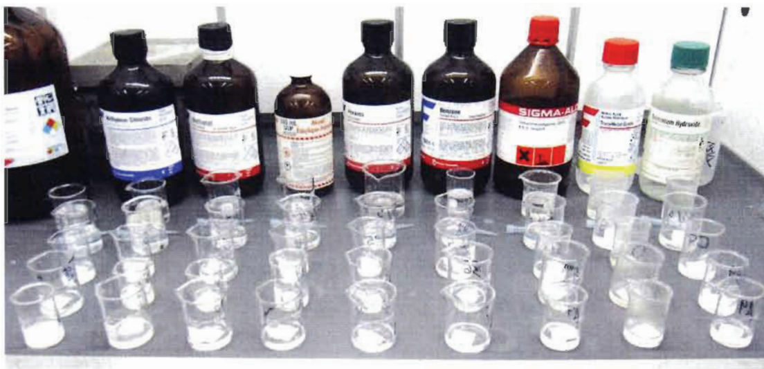
Figure 3-3. Experimental set-up in fume hood for chemical resistivity study.
