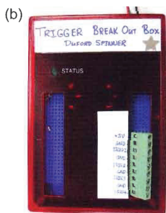
Figure 2-10. Trigger breakout box. (a) Circuit diagram, (b) Photograph of Stage v2.0 trigger breakout box. (c) Photograph of Stage v3.0 trigger breakout box.
