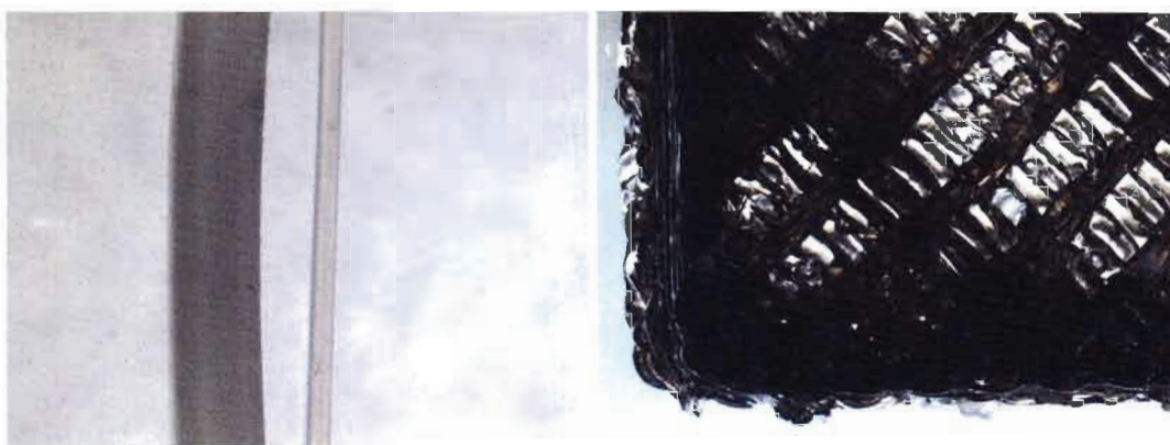
Figure C-5. uPrint ABS raw and extruded material (left) and “printed” support structure (right) at 16.8x magnification
