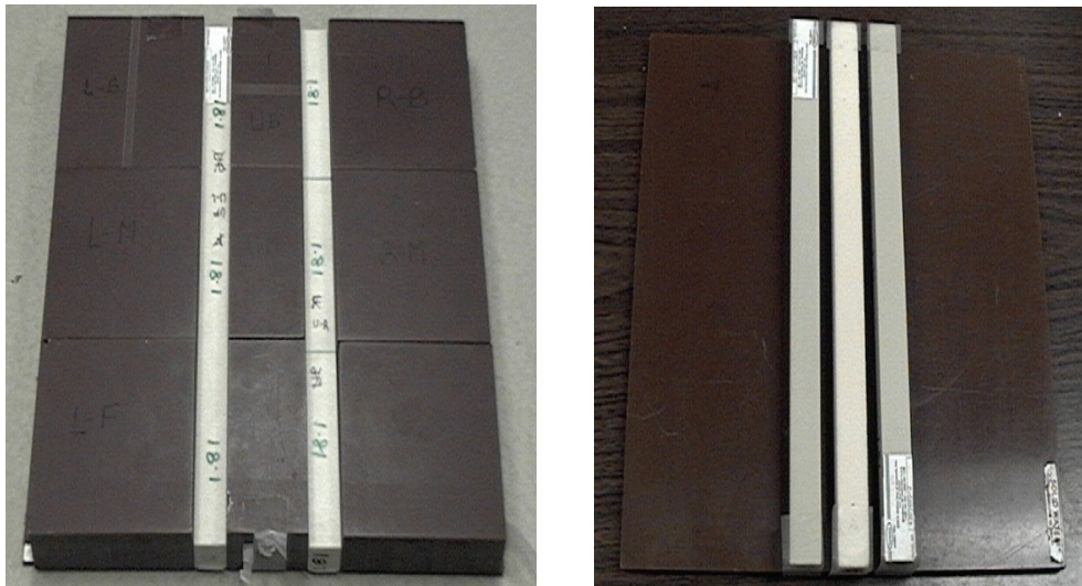
Figure 5.2: Physical phantoms used for measuring heterogeneity effects on dose profiles. On the left, a phantom with two heterogeneity bars (i.e., the “two-bars” phantom) sandwiched in solid water blocs; On the right, a phantom with three heterogeneity bars (i.e., the “three-bars” phantom) separated by air gaps.
