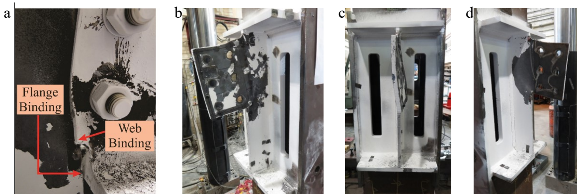
Fig. 5-9. Specimen BG3-2-13-F-200 : (a) binding between beam and shear plate, (b-d) deformed shape at end of test
