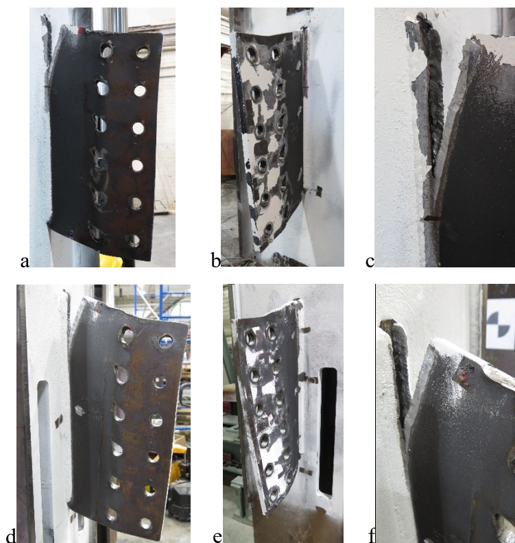
Fig. 7-8. Deformed shape of Specimens: (a-c) BC6-2-16, (d-f) BC6-2-16-500C
