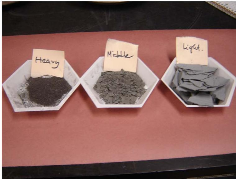
Fig. 7. Three gravity separated fractions: heavy, middle and light
