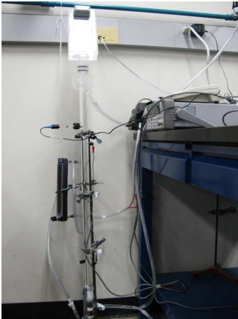
Fig. 13. Sedimentation potential apparatus for bubble swarms
