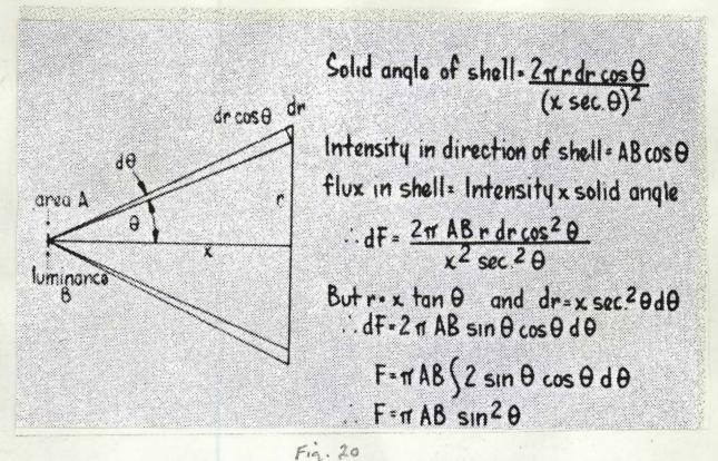
Calculating the flux radiated by a plane source into a hemisphere.
