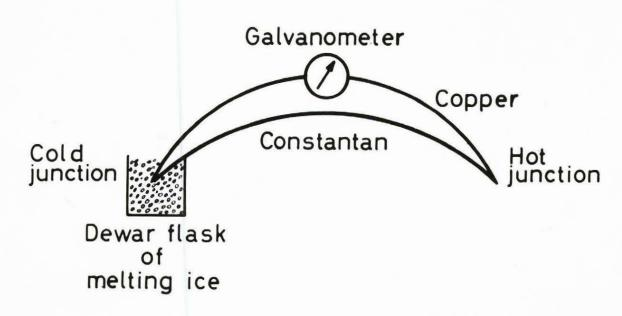
A simple thermocouple circuit
