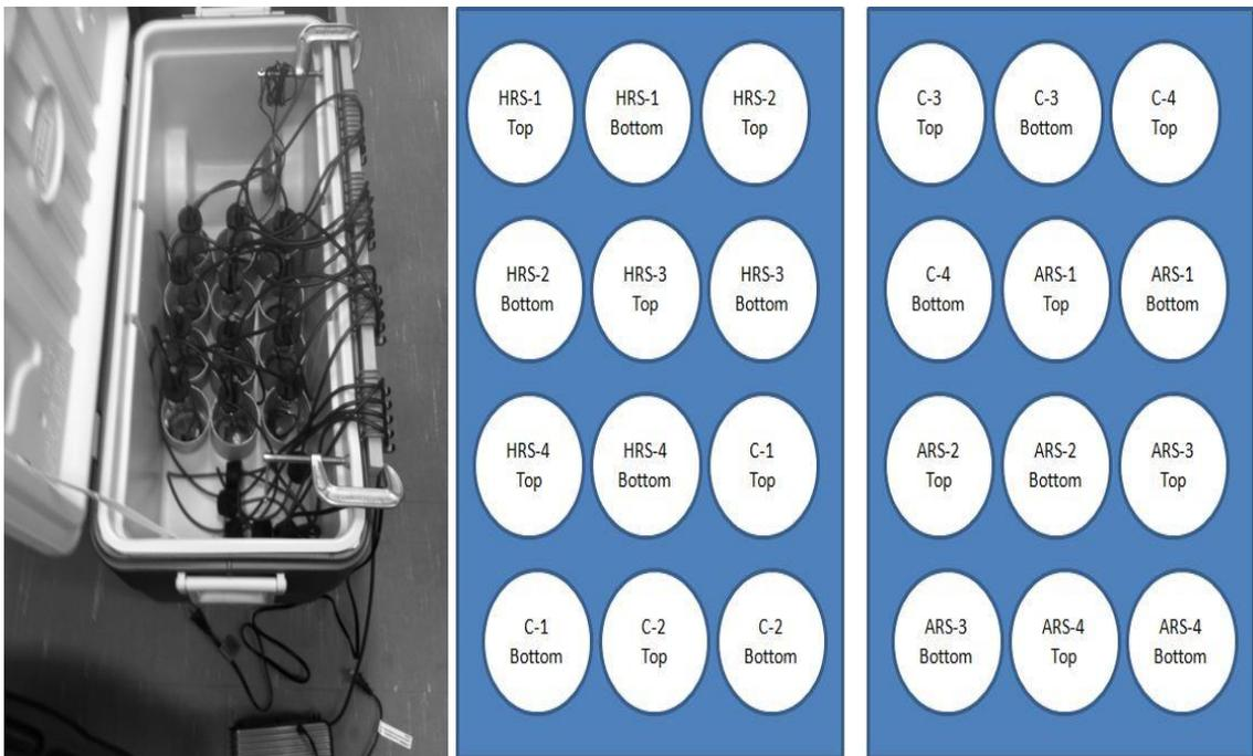
**Figure 13: Water bath with aeration lines being assembled. Two baths are used. On the right side, the layout of the flasks can be found.**
