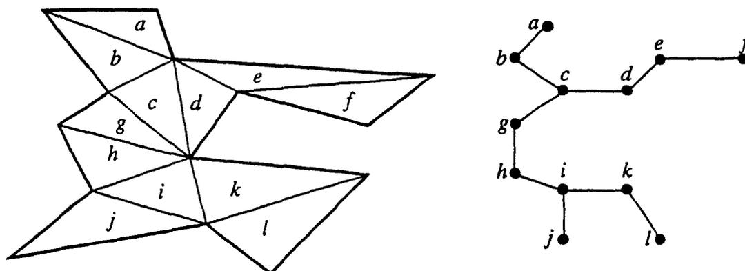
Figure 1.9: A triangulation and its dual tree
