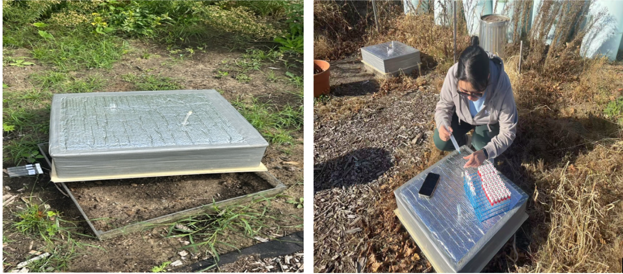
Figure 13. Manual Non-Steady-State Chamber Setup for Soil Greenhouse Gas Flux Measurements (left). The author is taking the sample (right).
