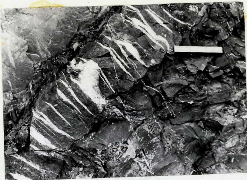
Figure 32. Calcite-filled conjugate joints restricted to an 8 in. thick limestone layer. A few quartz-filled fractures cut across them. The scale is 6 in. long.
