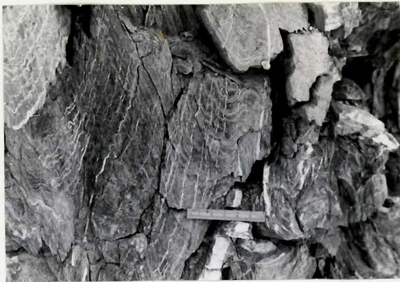
Figure 30. Quartz-filled fractures on Face # 3. Scale is 6 in.
