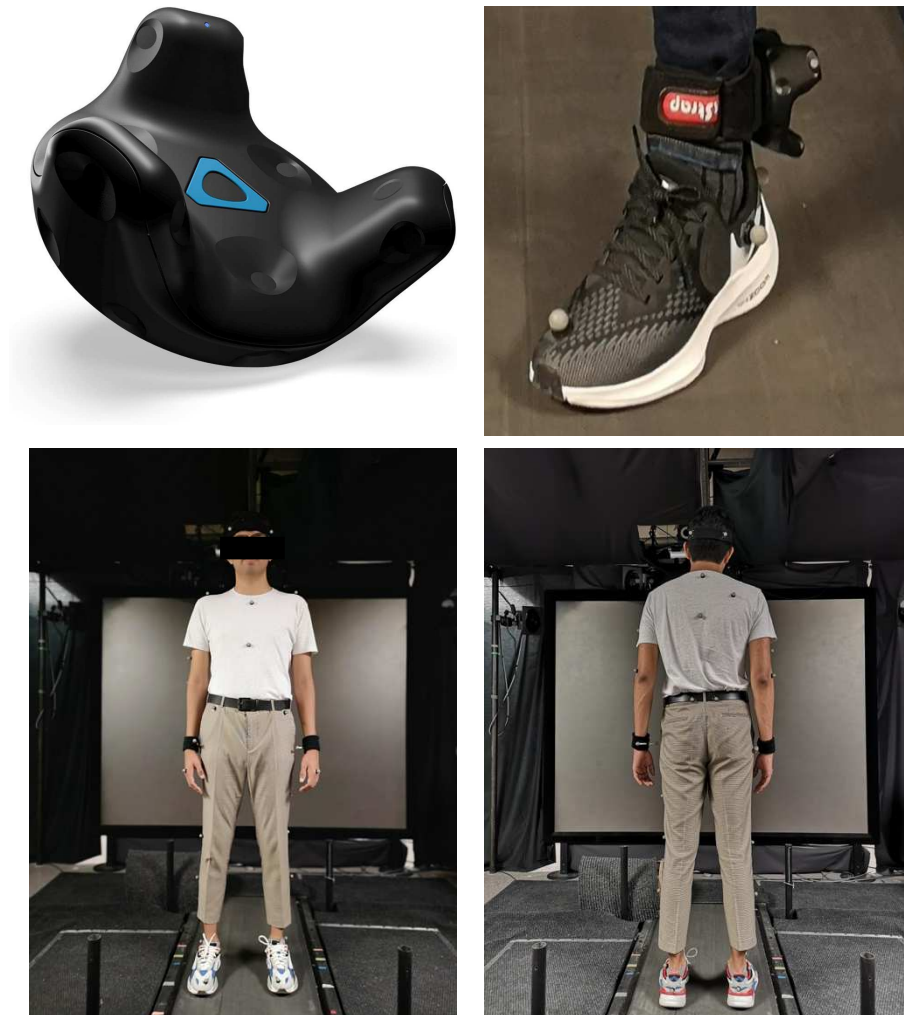
Figure 7.1 Top left: a tracker device from VIVE™ used for the foot strike detection. Top right: The placement of the tracker device (around the ankle) during the experiment. Bottom: The 14 mm pearl hard markers placed on a participant based on the plug-in gait model (left: back view; right: frontal view). The participant is standing on a self-paced treadmill.
