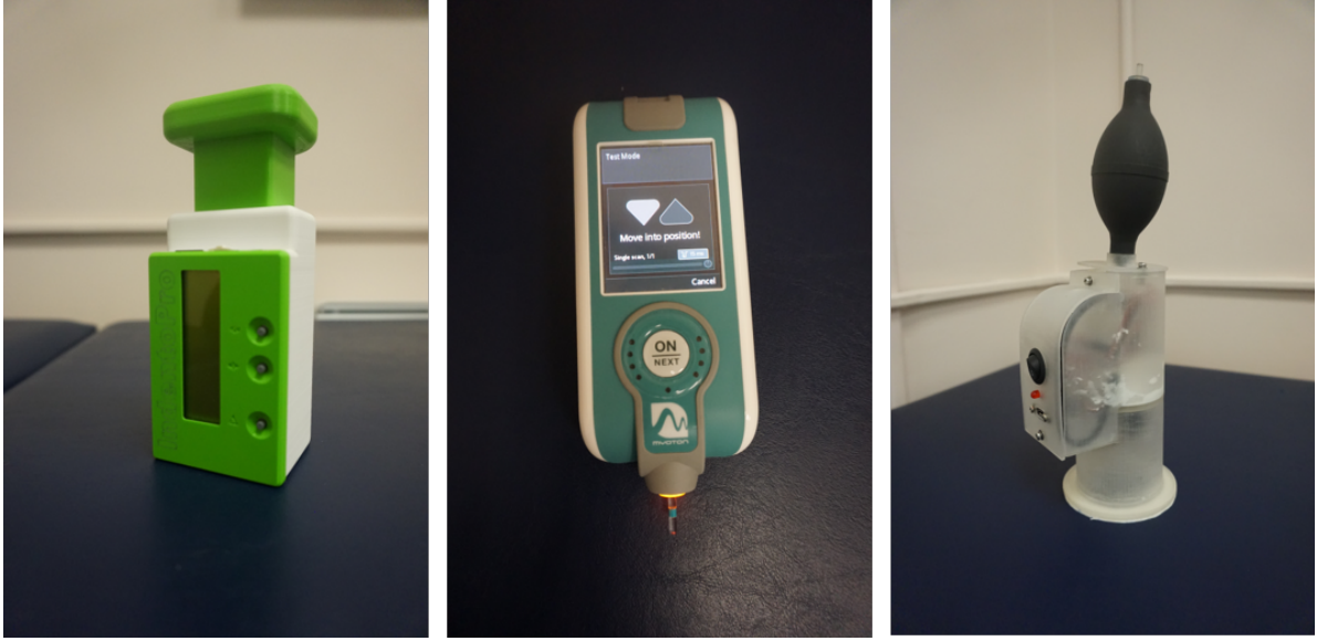
Figure 4.2.1: From left to right: IndentoPro (standard indentometer), MyotonPro (popularized myometer), and novel device.
