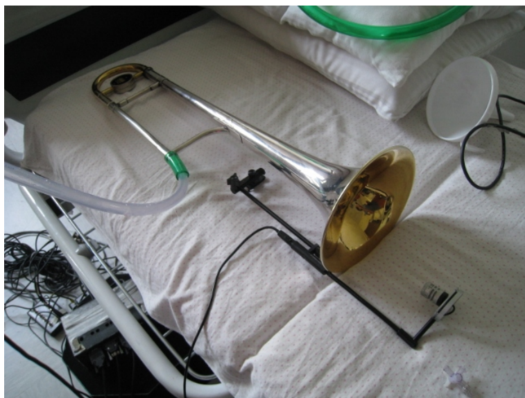
Figure 6.3 Experimental setup for recording of the radiated sound.
