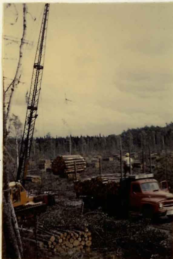
PHOTO 14 'Yarder' at work in highly mechanised company exploitation of the Clay Belt Forests.
