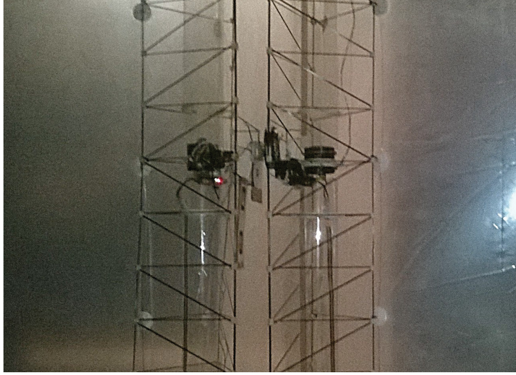
Figure 6–2: Target(left) and chaser(right) Tryphon in docked position with docking mechanism contact at UQAM’s Studio-théâtre Alfred Laliberté
