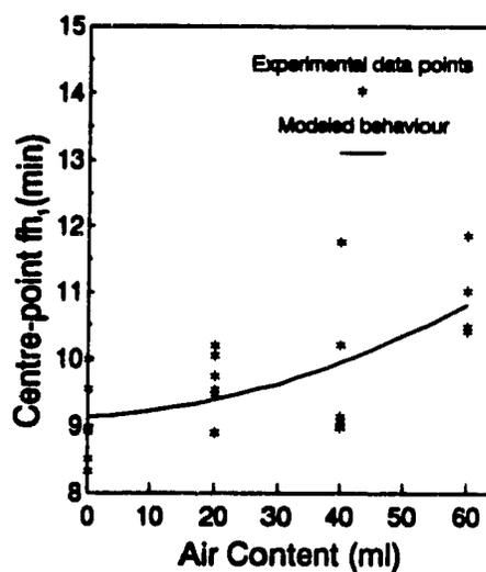
Figure 14. Centre-point  $f_h$  values vs. air content for test bricks in retort pouches for second region of heat penetration curves ( $f_{h2}$ ).
