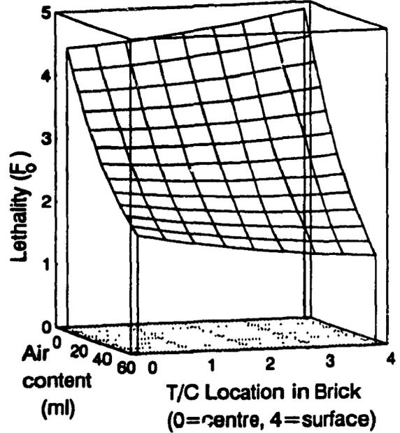
Figure 21. Location of lowest overall lethality (cold spot) as a function of entrapped air content for heating + cooling for the four processing conditions.
