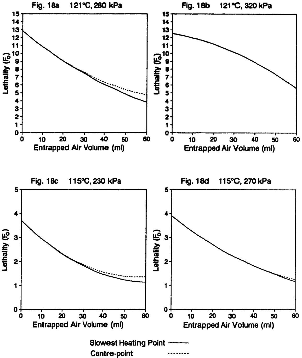
Figure 19. Cooling lethality as a function of both entrapped air content and location of thermocouples in the test bricks at each of the four processing conditions.
