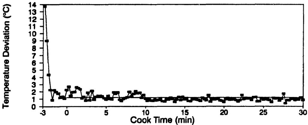
Figure 6. Temperature response for two locations during sample runs in the three retort systems operating at 121°C and 280 kPa.
