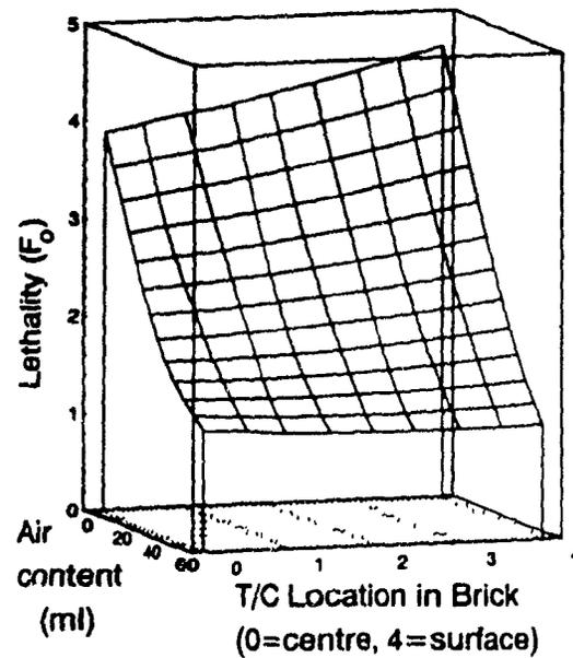
Figure 17. Location of slowest heating region as a function of entrapped air for 30 minutes of heating (cooling excluded) for the four processing conditions.
