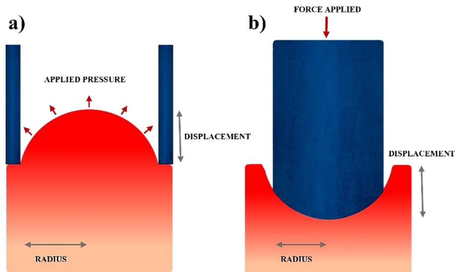
Figure 2-3 Characterization of soft tissue undergoing a) suction and b) indentation/myotonometry.
