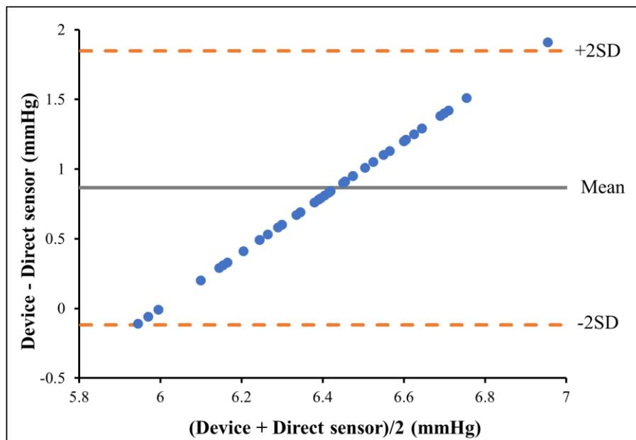
*Figure 3-8 Bland and Altman analysis comparing the internal pressure measurement using the device against the direct pressure sensor measurement.*
