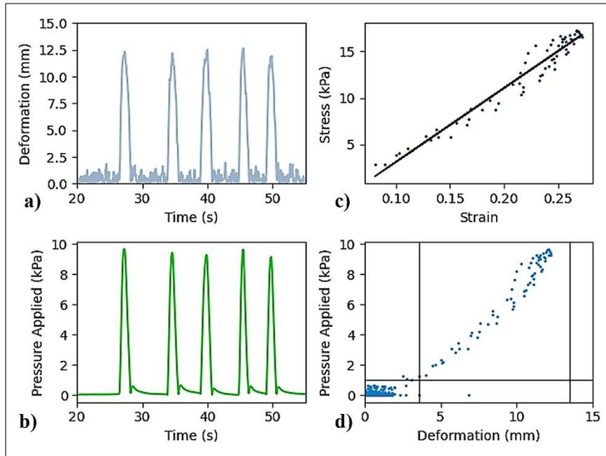
Figure 4-2 Device measurement results. a) Material deformation. b) Pressure pulses applied. c) Stress-strain diagram and average elastic modulus. d) Discretization process showing the pressure-deformation relationship.
