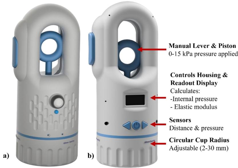
Figure 3-1 Evolution of novel non-invasive suction device. a) Early version, including ON/OFF button. b) Improved device configuration that features a display for presenting measurement data and navigation buttons.
