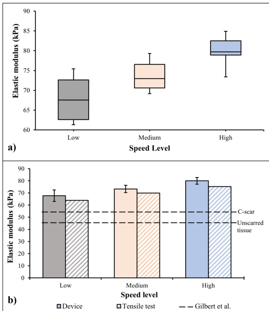
Figure 3-7 Elastic modulus results at different strain rates. a) Device results. b) Elastic modulus validation.
