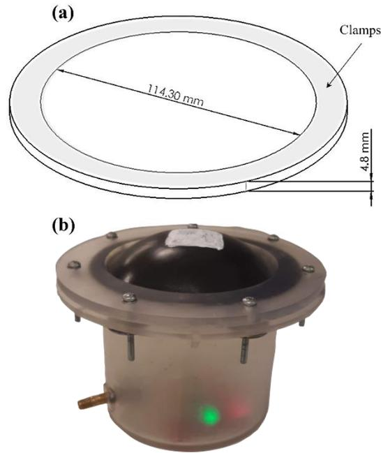
Figure 3-3 The benchtop model. a) The sample dimensions. b) Picture of model.
