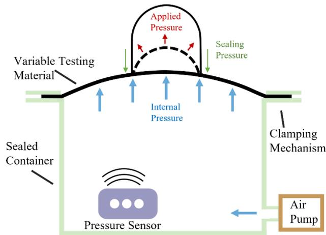
*Figure 3-4 The benchtop model diagram depicting the position of the novel suction device, the displacement of the material during measurements, and the directions of the internal and sealing pressures.*
