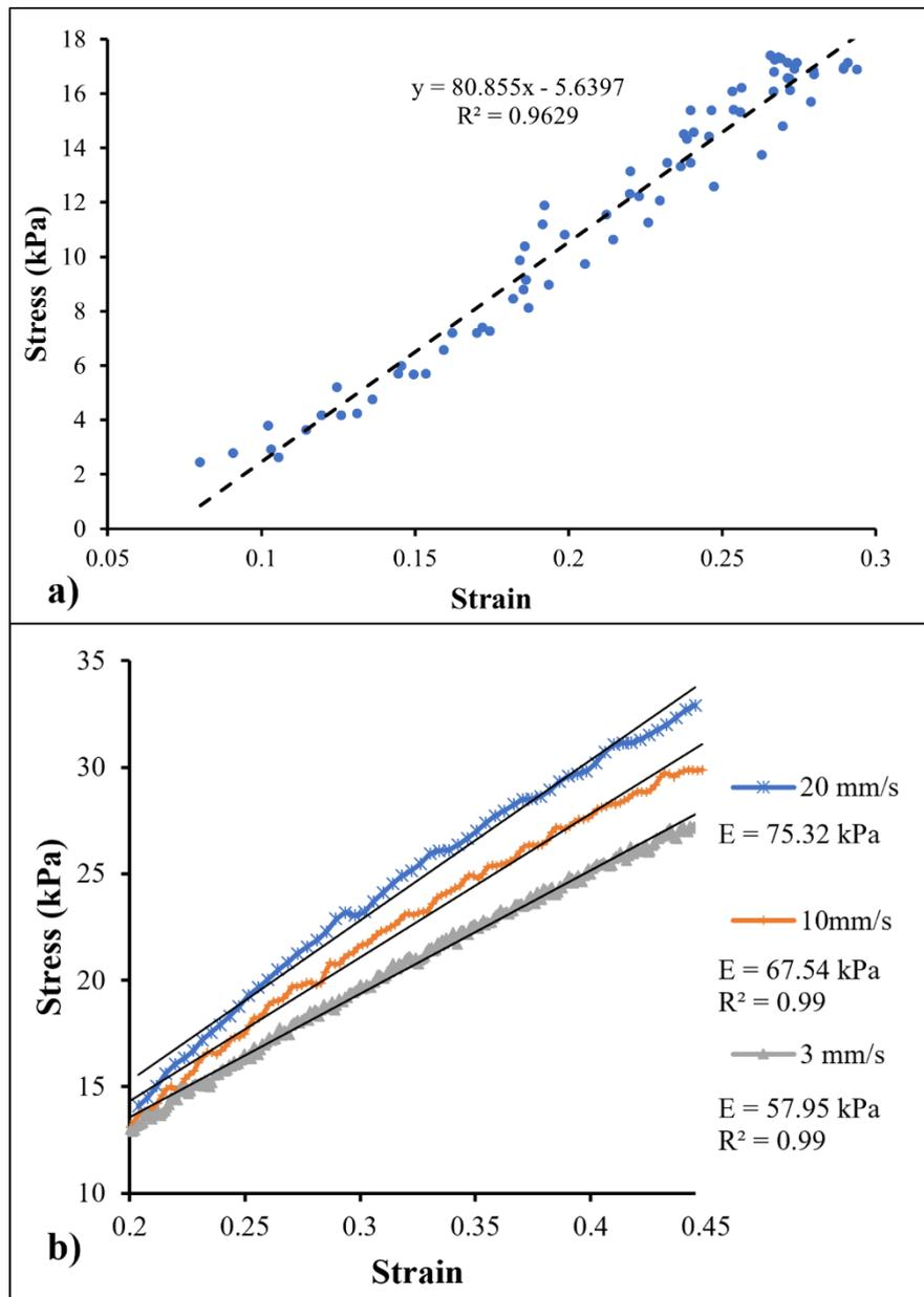
Figure 3-6 Stress-strain diagram and elastic modulus calculation for the rubber phantom material. a) Example of the device measurement at the high strain rate. b) The tensile test results, including 20% pre-strain, to validate the phantom mechanical behavior at 3, 10, and 20 mm/s.
