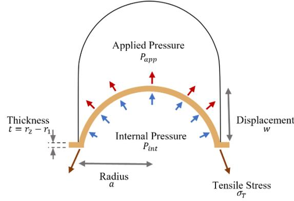
Figure 3-2 Diagram of theoretical design and formulation variables.
