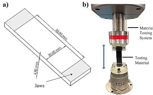
Figure 3-5 The tensile test. a) The sample dimensions. b) The tensile test machine setting.
