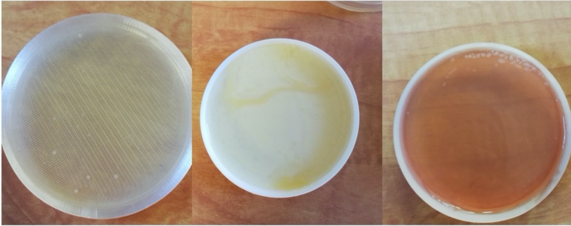
Figure 2: Examples of contamination on 3D-printed dishes following 70% ethanol cleaning (standard 2 x 1 min soak). From left: PLA, ABS, SG resin. Contamination severity was highly variable, ranging from small isolated colony(ies) (left) to colonies covering half the plate (middle).
