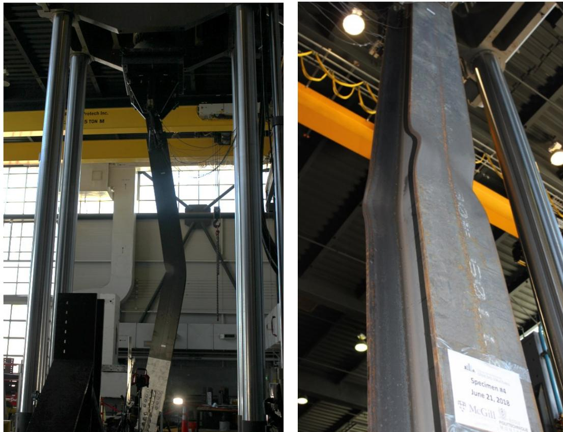
*Figure 4-40 Global and local buckling of the W-shape brace of specimen C360-C*
