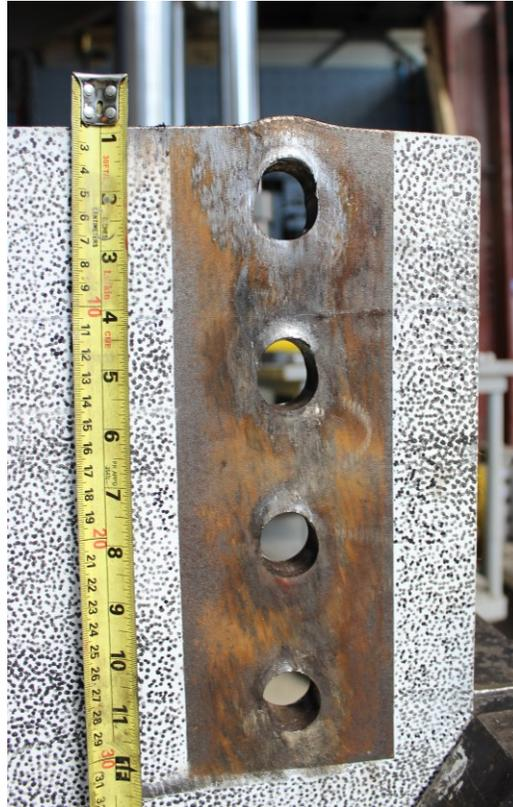
*Figure 4-49 Deformation beyond the edge of the bottom gusset plate of specimen C360-C*
