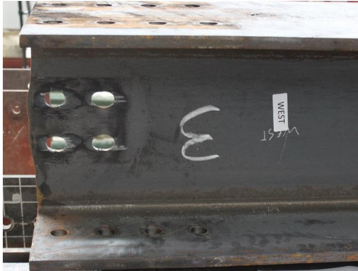
Figure 4-43 Deformed W-shape web of top connection in specimen J360-T
