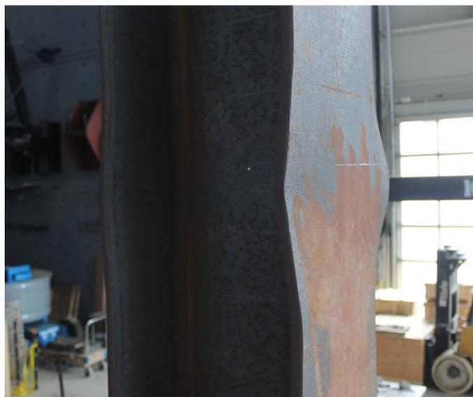
Figure 4-23 Local buckling in middle of W-shape of specimen J310-C
