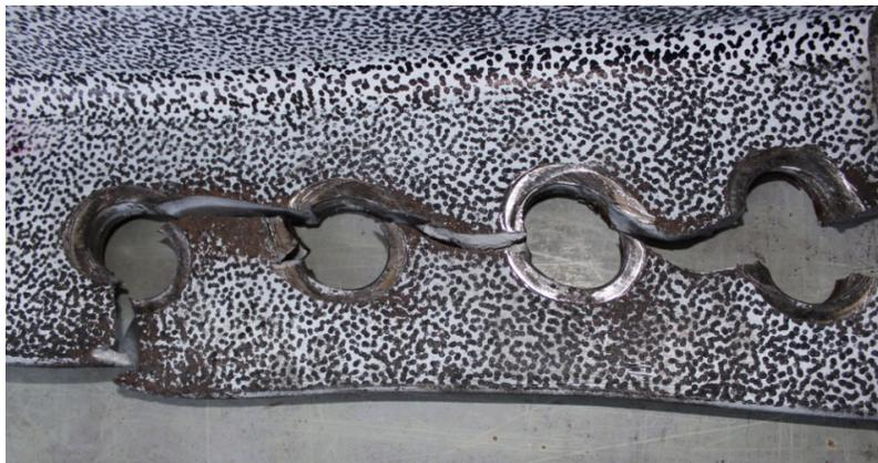
*Figure 4-45 Block shear through net shear area in angle*
