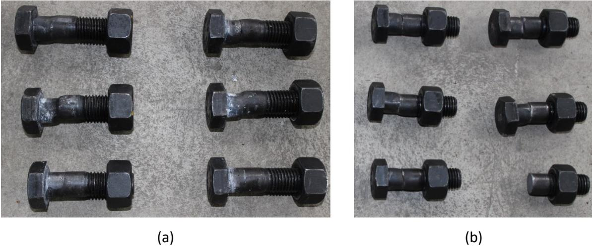
Figure 4-21 Bolts from J310-C (a) bottom flange connection (b) top flange connection (sheared)
