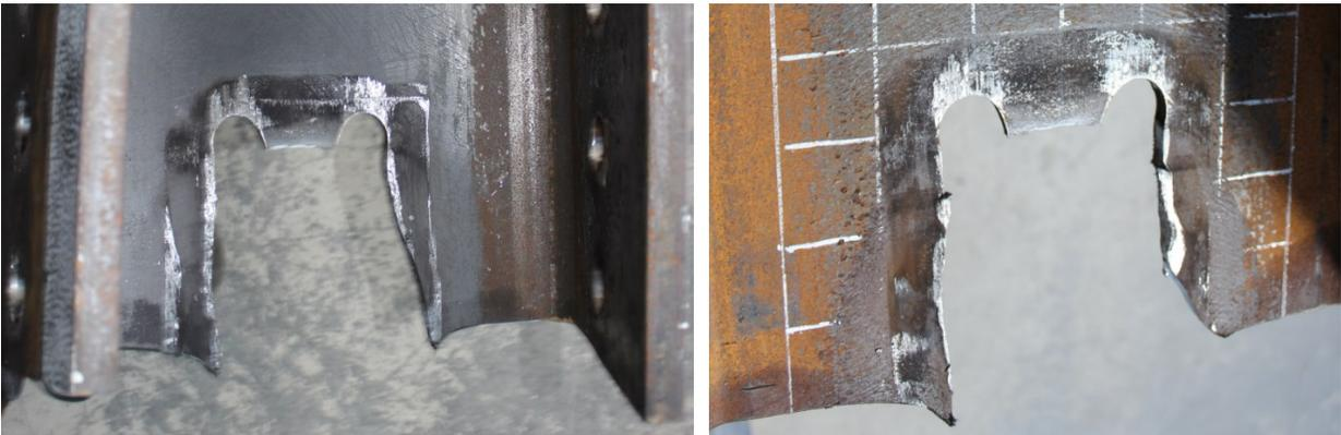
Figure 4-42 Block shear in the W-shape webs for specimens: (a) C360-T and (b) C360-C
