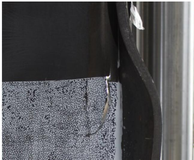
*Figure 4-31 Locally buckled flanges and torn web in specimen J360-C*
