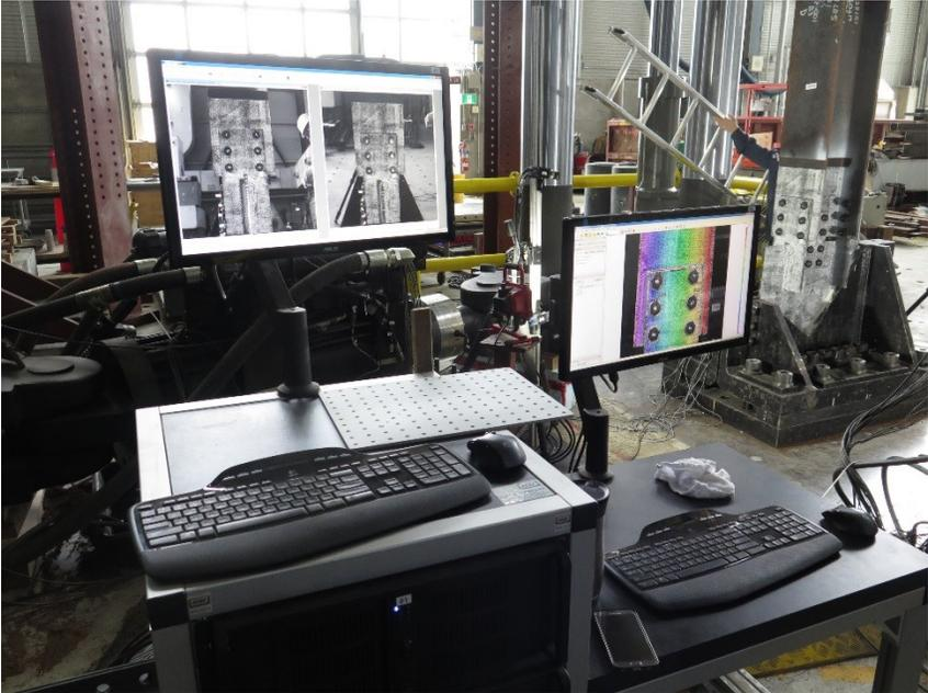
Figure 4-13 DIC control setup showing views (on monitors) of the three camera angles
