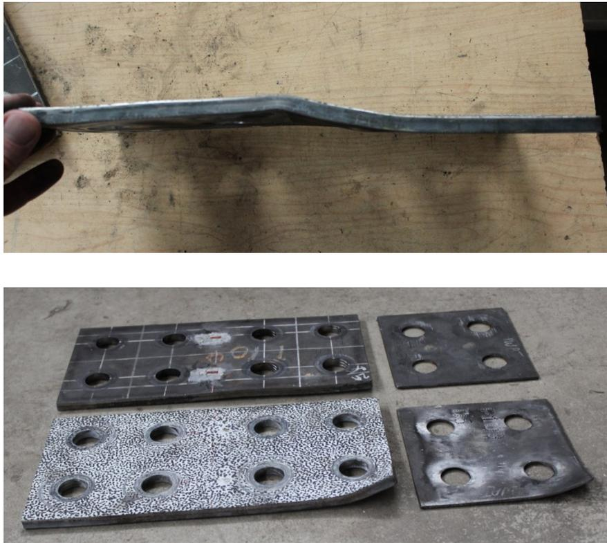
*Figure 4-34 Photos of deformed web plates*
