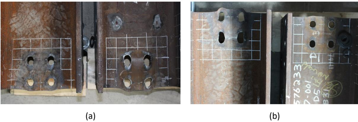
Figure 4-22 Deformed W-shape webs of J310-C on the left and J310-T on the right: (a) bottoms of W-shapes (b) tops of W-shapes
