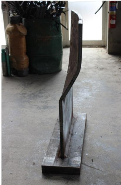
Figure 4-44 Post-test bent bottom gusset plate from specimen C360-T
