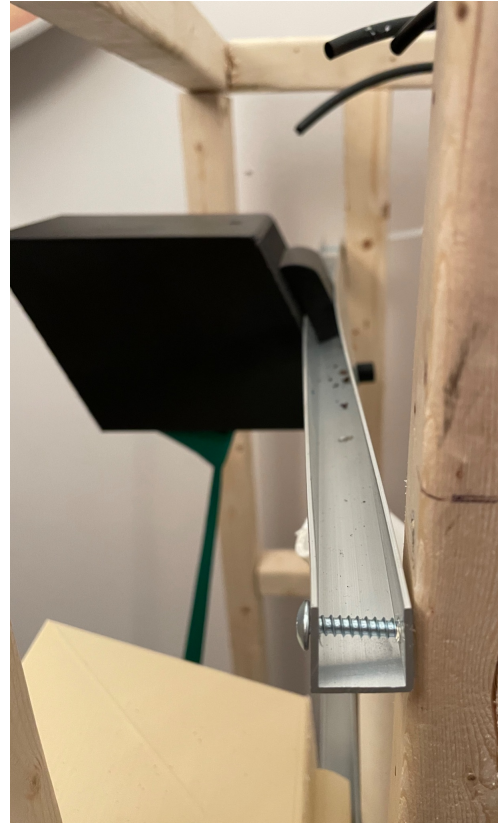
Figure 17: Visible bending of U-Channel
