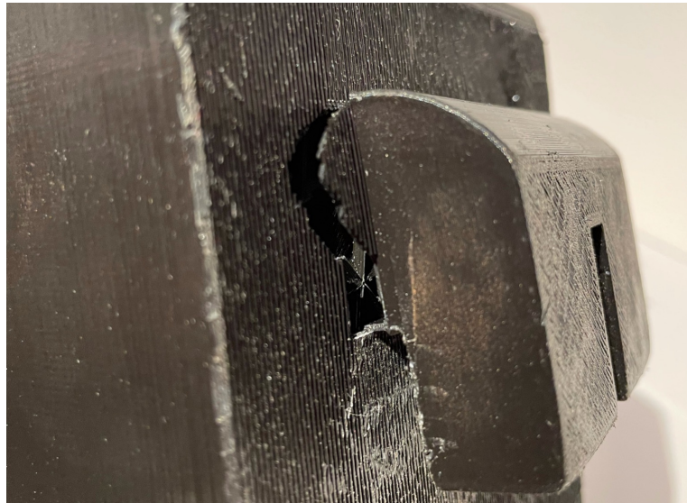
Figure 18: Damage to clip after testing with 35 pounds of weight
