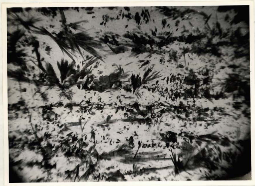
FIG. 8 40 X Alteration of chlorite to anthophyllite.
