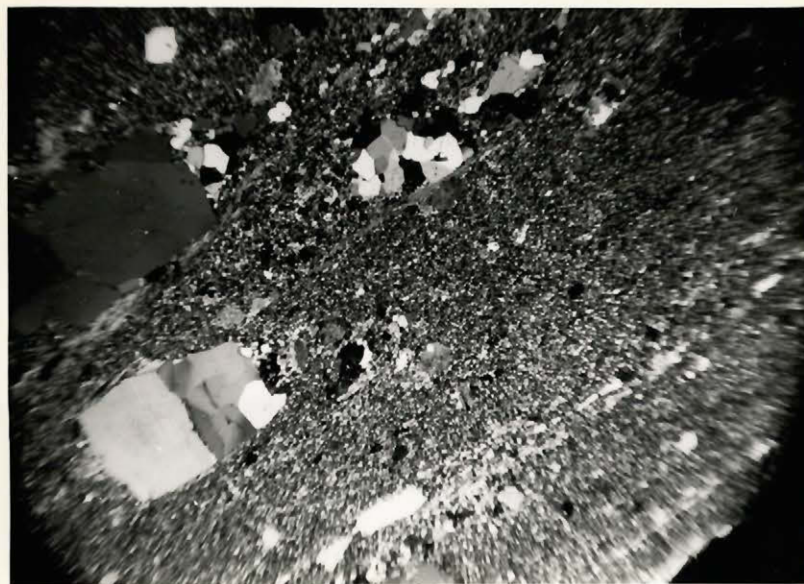
FIG. 6 40 X Texture and Structure of Quartz Sericite Schist. (Crossed Nicols)
