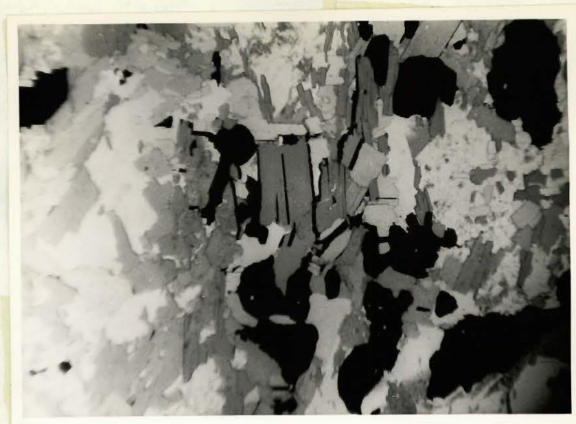
FIG. 17 40 X Replacement of biotite by sulphides
