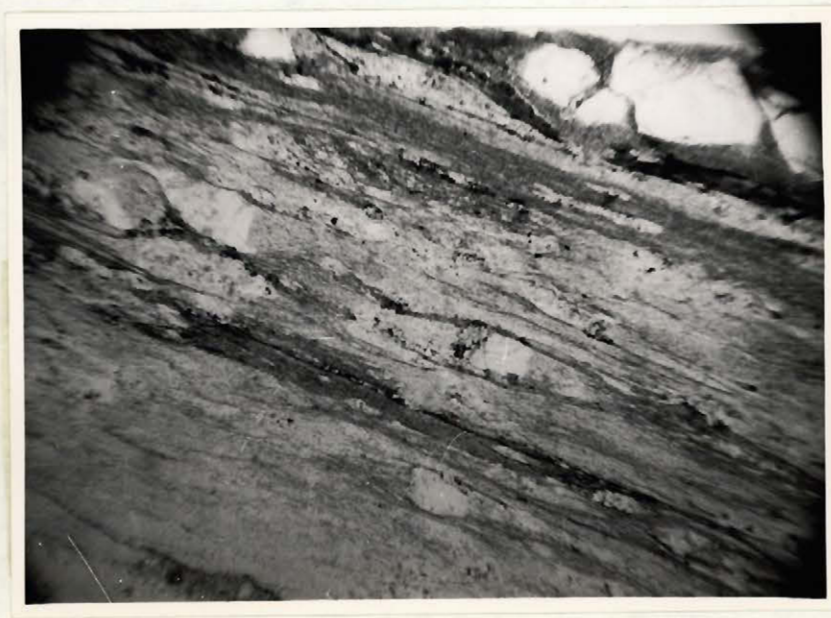
FIG. 4 40 X Texture and Structure of Quartz Sericite Schist.
