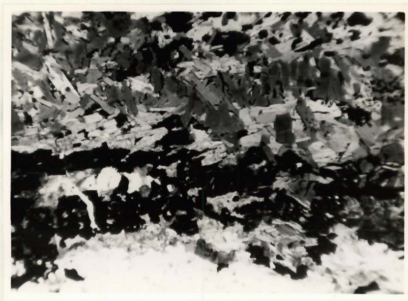
FIG. 18 40 X Sulphides beginning to replace a biotite inclusion.
