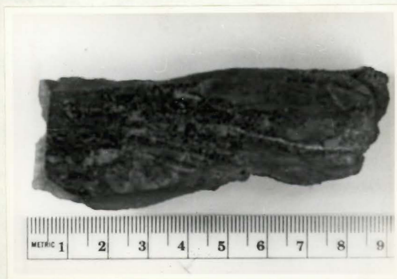
FIG. 3 Polished section of a breccia, the particles being surrounded by chlorite.
