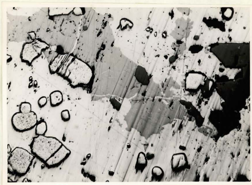
FIG. 27 40 X Age relationships of pyrite, chalcopyrite and sphalerite.
