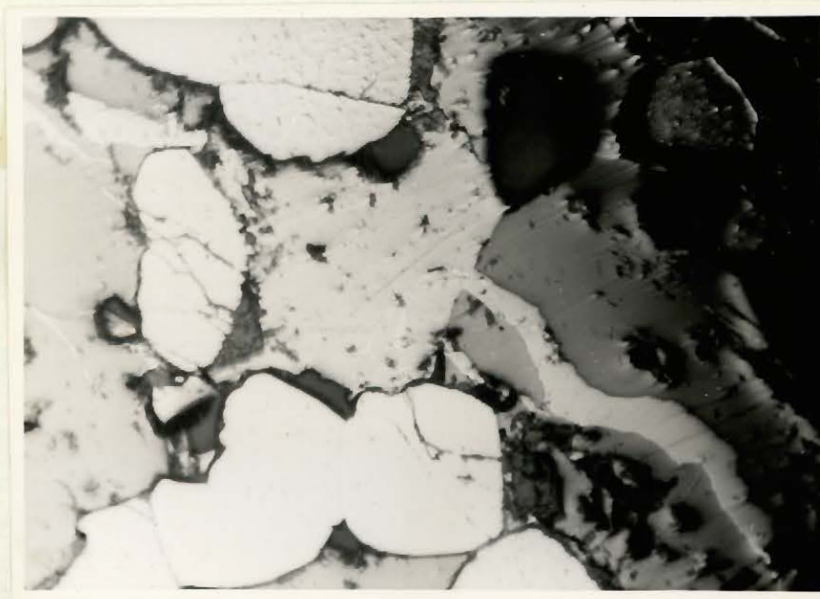
FIG. 26 80 X Fracturing of the ore minerals.
