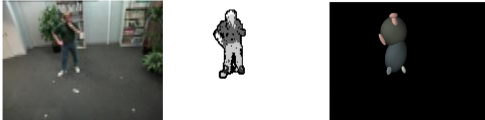
Figure 2–1: The Pfinder system [86]: The left image shows the initial camera view, the middle image shows the segmented user (based on background removal), and the right image shows a rendering of the blobs that make up the tracked human figure.
