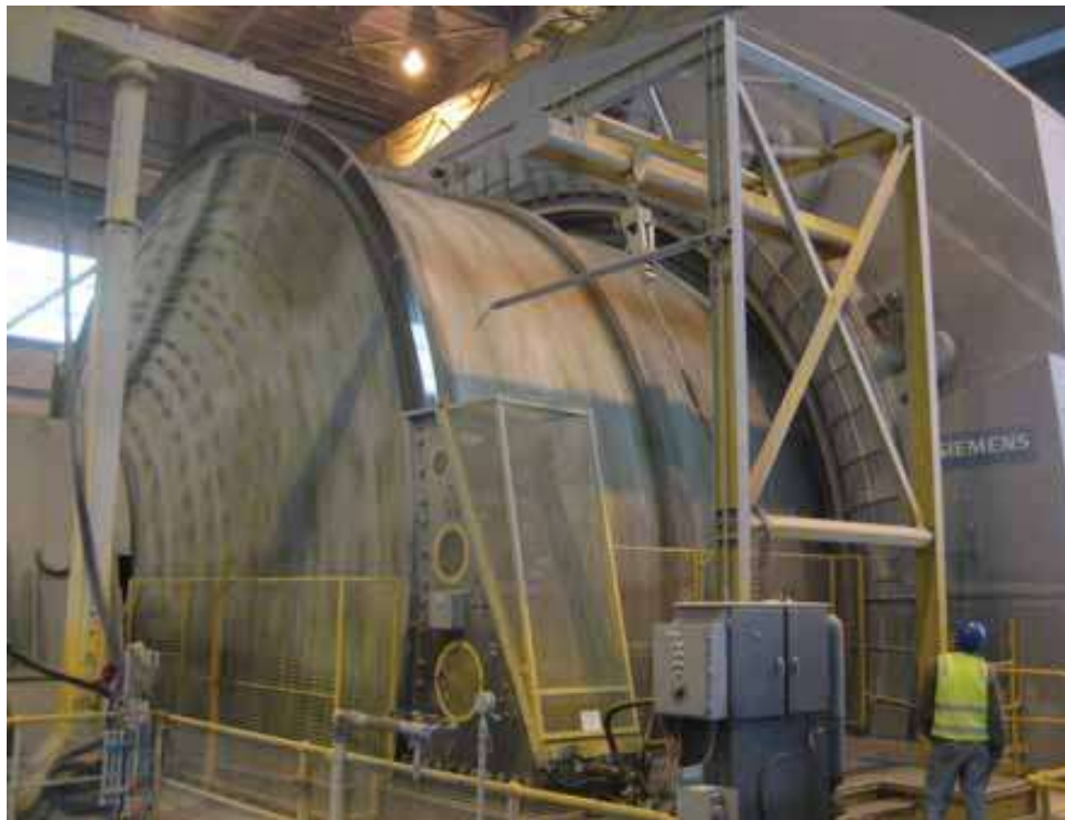
Figure 2.3: A 40 ft SAG Mill in Operation (Courtesy of Norcast Wear Solutions)
