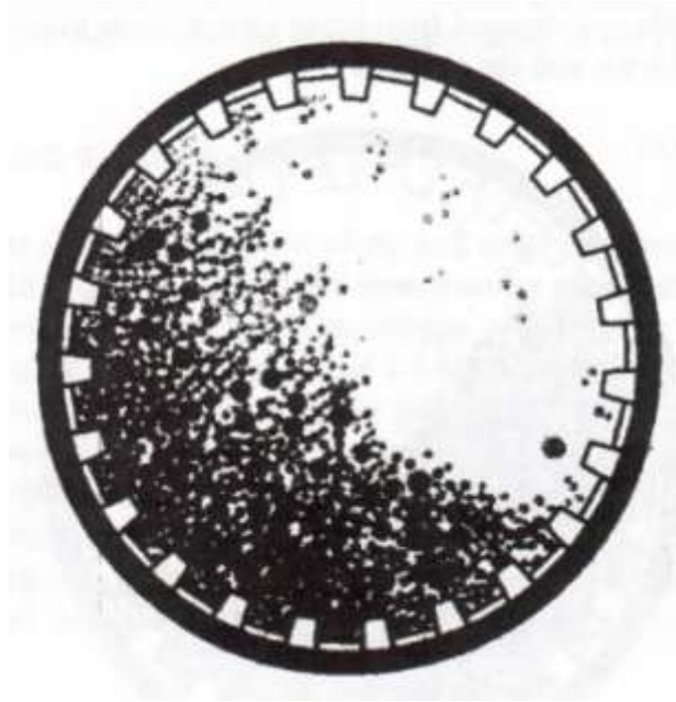
Figure 3.9: Materials Fill-Up Level of Grate-Discharge Grinding Mill (Cleary 1998)
