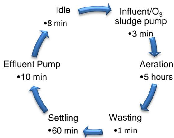
**Figure 10.** Six hour sequencing batch reactor cycle. All processes occur within the same container and only the operational conditions change between phases.
