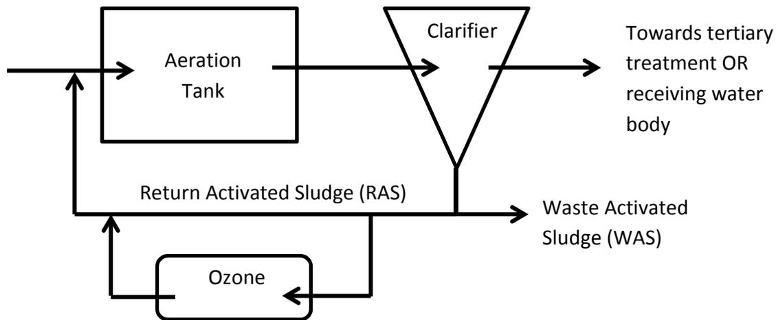
**Figure 2.** Schematic of a typical activated sludge wastewater treatment plant including a typical location for ozone application
