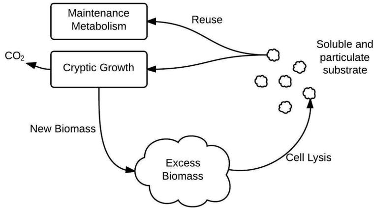
**Figure 4.** Schematic diagram of cryptic growth, one of the proposed mechanisms that contribute to excess biomass reduction. Non-biodegradable biomass is solubilized by the ozone and fed back to the reactor. A portion of the carbon is released as  $\text{CO}_2$
