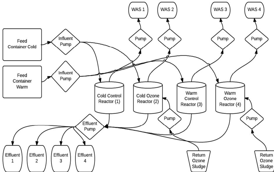
**Figure 9.** Full set-up schematic, showing the flow of the influent to the reactors, and the effluent from the reactors to individual containers. Also shown is the flow of mixed liquor from the reactors to the WAS containers, where a portion of it for the experimental reactors will be ozonated and returned to the reactors
