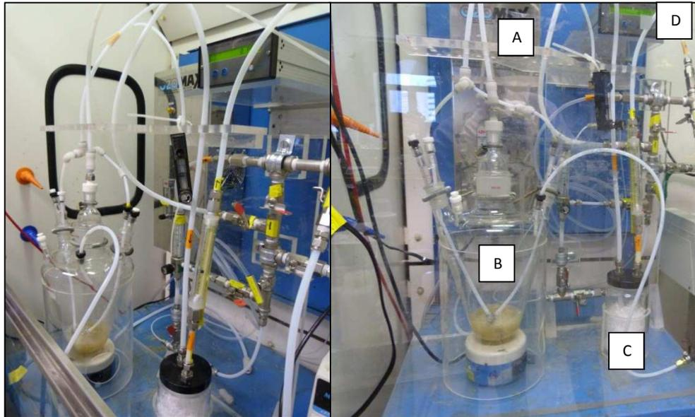
**Figure 11:** Lab batch ozonator showing (A) ozone generator, (B) biomass contactor, (C) solids trap, (D) residual ozone gas reader. Mixed liquor is placed in the contactor and ozonated for a predetermined time to achieve desired ozone
