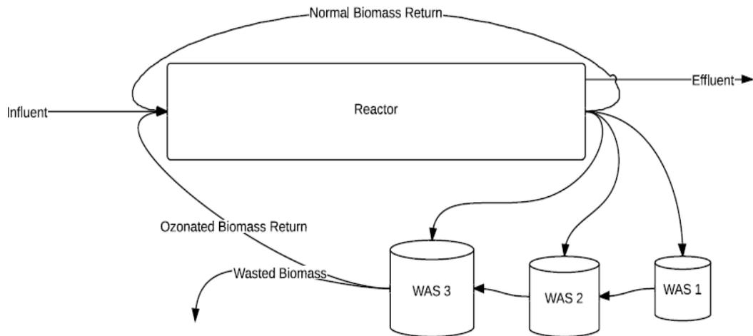
**Figure 12.** Simplified model diagram of ozonated reactor wasting layout. Three wasting containers with an HRT of 1 day were used to simulate the daily wasting and ozonated return of large volumes of mixed liquor.
