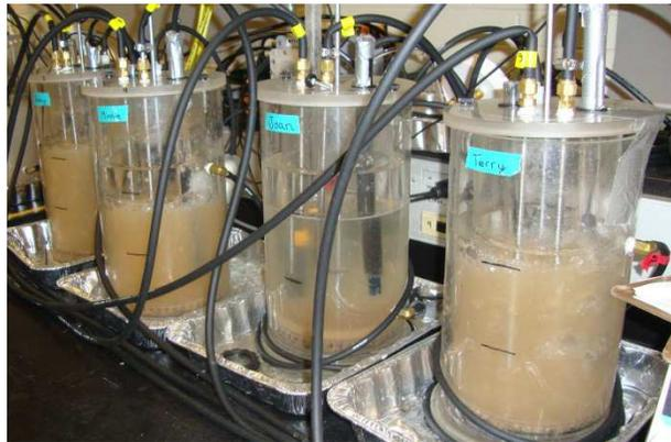
**Figure 8.** Photograph of reactors in operation. Note the third reactor is in the settling phase while the others are in the aeration phase.
