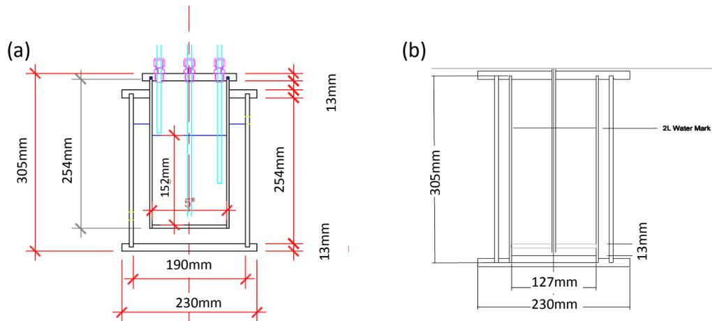
**Figure 7.** Initial (a) and final (b) reactor schematics. The main difference is the placement of the inner cylinder. In the final design, the inner cylinder is resting on the bottom rather than suspended. This simplifies the design allowing for a single layer lid.
