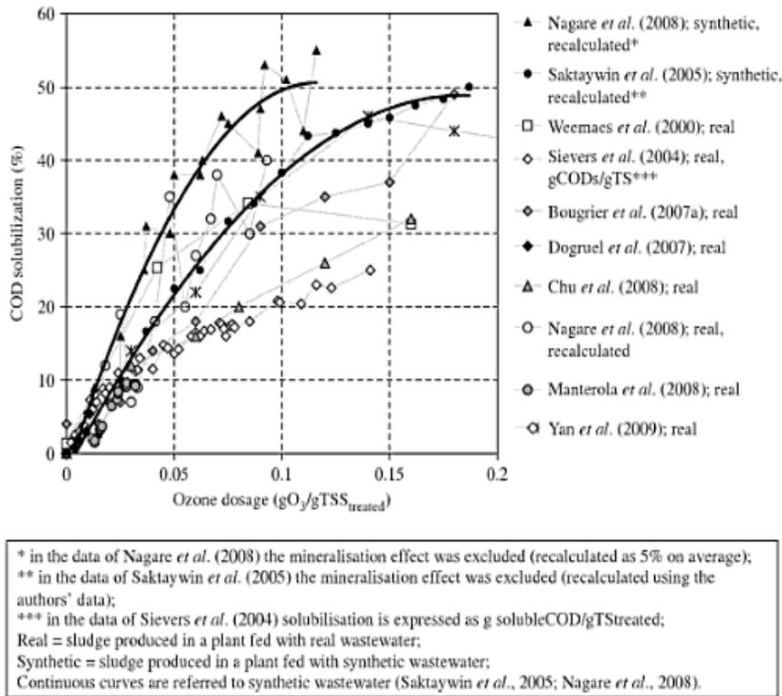
**Figure 3.** COD solubilization percentage as a function of ozone dose over total solids compiled from multiple studies. Although all use different types of biomass and have slightly different slopes, the general shape of the curve is similar in all. (Foladori et al. 2010)
