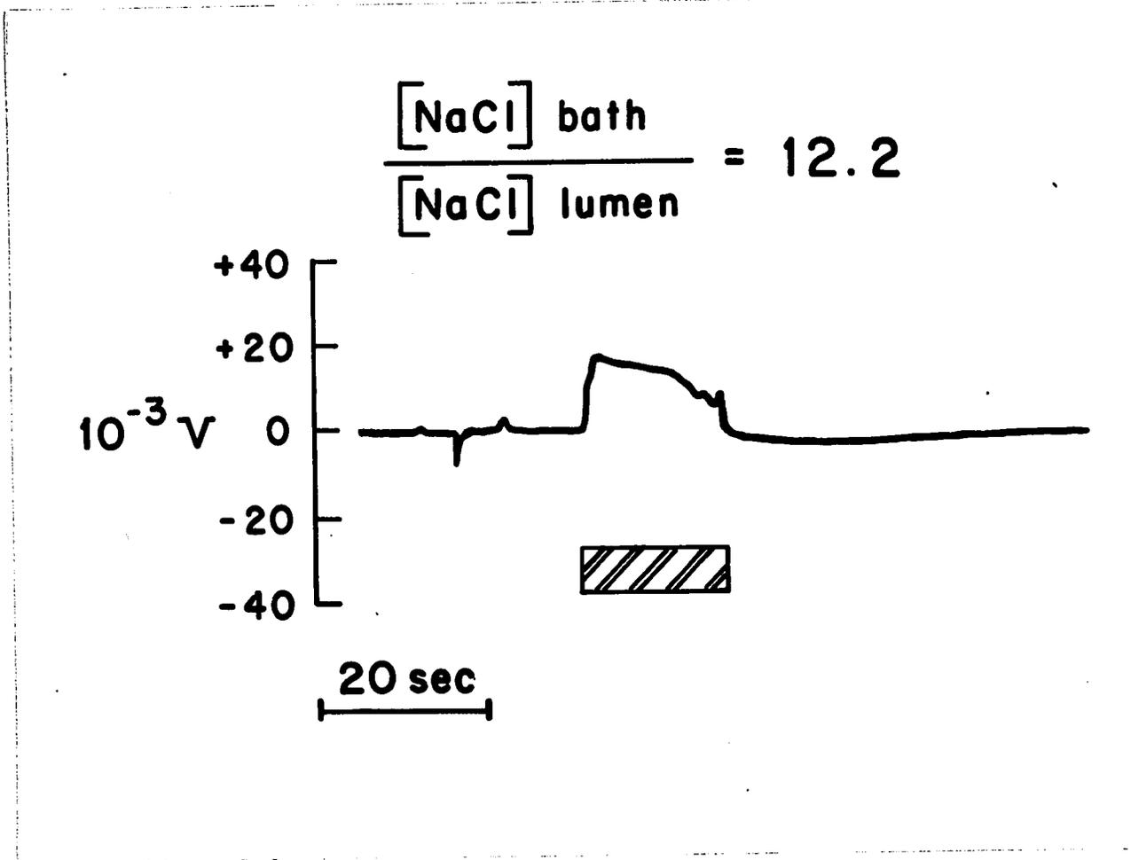
Figure B-6: Tracing from a representative salt gradient experiment. Penetration into the lumen is indicated by the initial downward deflection. The lumen was perfused for an interval corresponding to the hatched bars with a test solution in which NaCl was partly substituted by sucrose.
