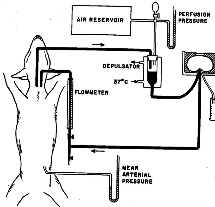
Figure B-1: Diagram of circuit for isobaric auto-perfusion of the dog kidney. Arterial blood from the carotid passes through a depulsator at 37 C connected to a damping reservoir maintaining a constant perfusion pressure. The isolated kidney is embedded in agar, leaving a small area on the surface accessible for micropuncture. Renal venous blood returns through a rotameter to the jugular vein.
