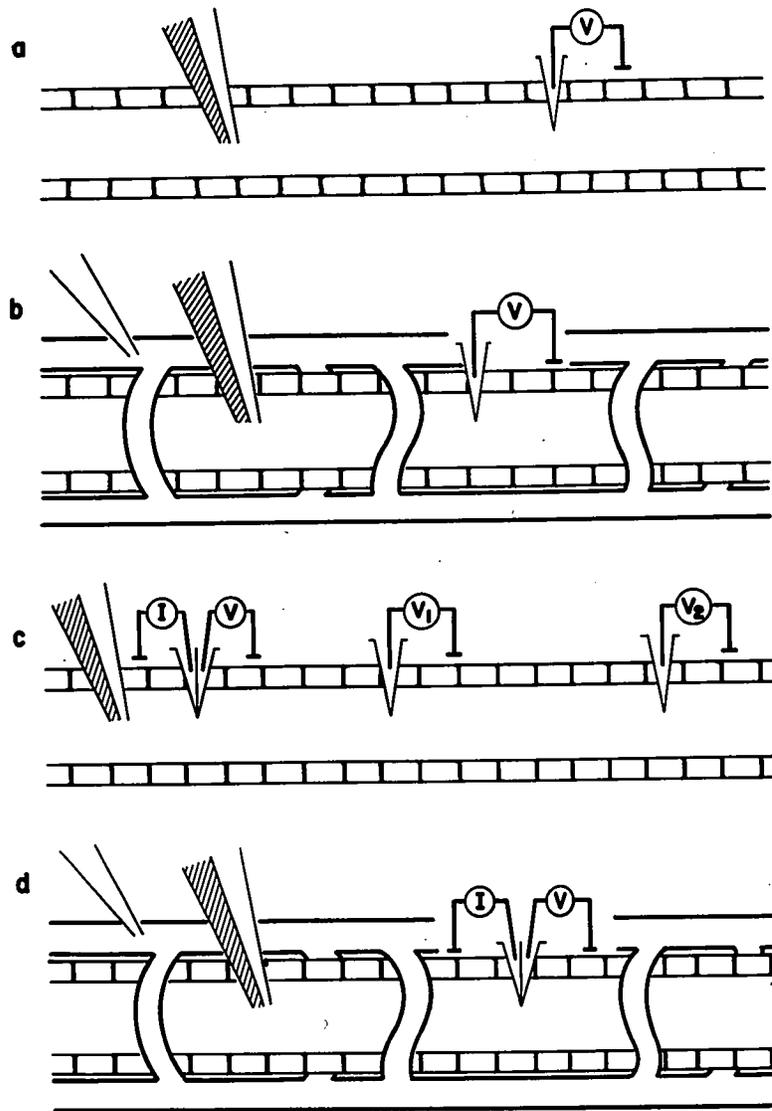
Figure B-2: Methods used for microperfusion of proximal tubules and peritubular capillaries, and for measurement of transepithelial potential differences and resistances. (See text for explanation).
