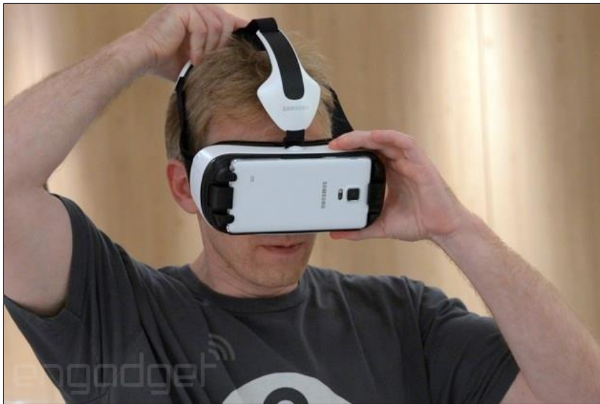
Figure 46, A Samsung smartphone works as a removable display in Samsung's new VR headset. [Source: "How Samsung's VR headset convinced John Carmack to join Oculus VR" (Gilbert 2014)]
