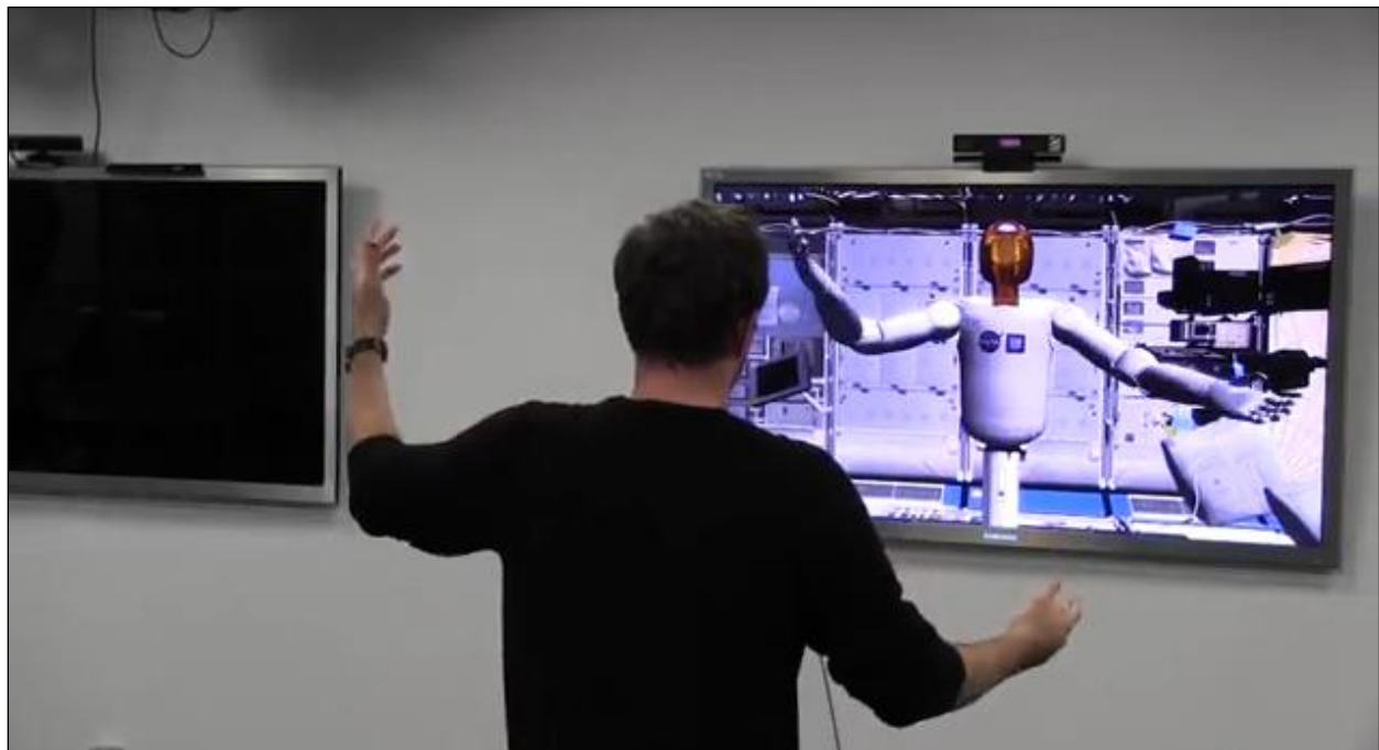
Figure 22, A mirror-mapped demonstration involving a virtual version of NASA's Robonaut 2. [Source: "NASA Robot Arm Control with Kinect" (NASA 2013)]
