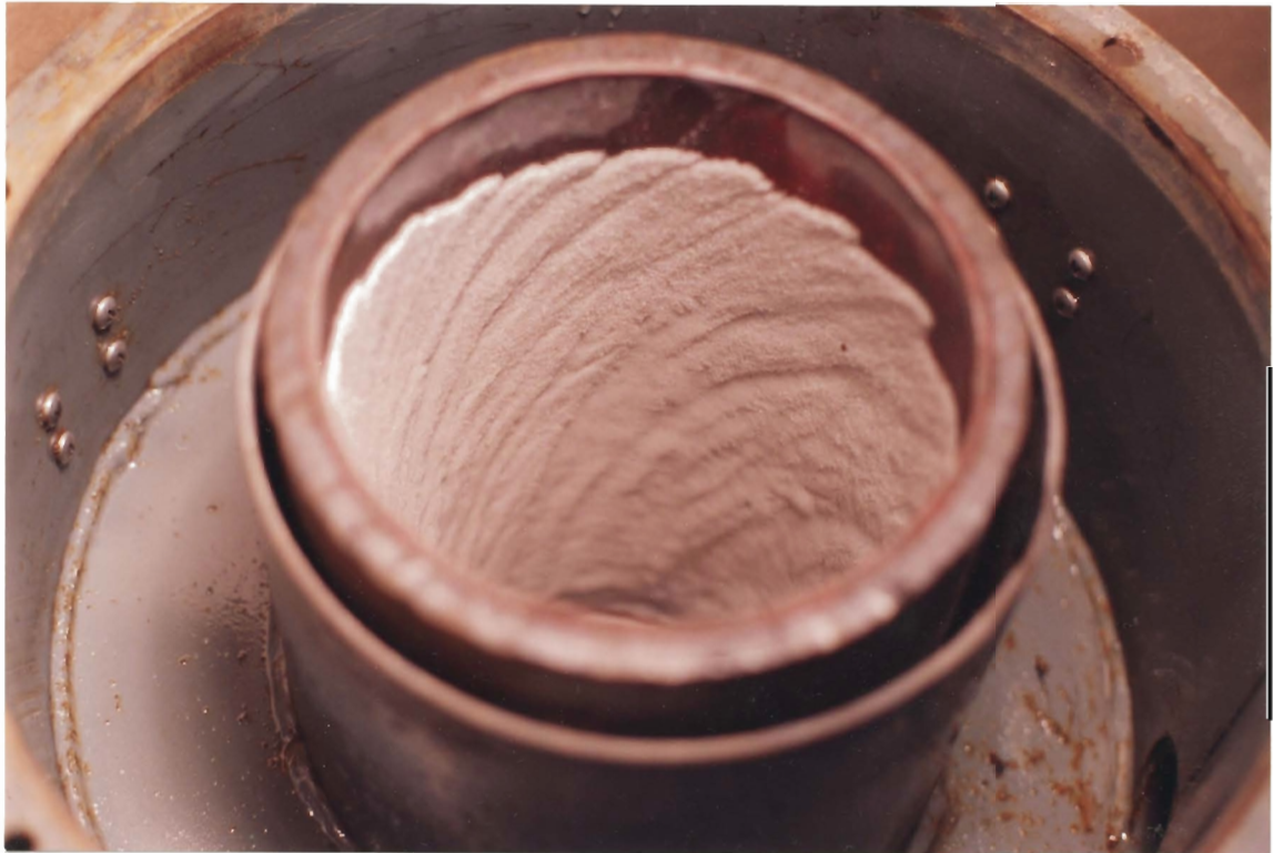
Plate A: Concentrate Bed after 10 seconds of Falcon Operation (Feed: Silica/Magnetite)
